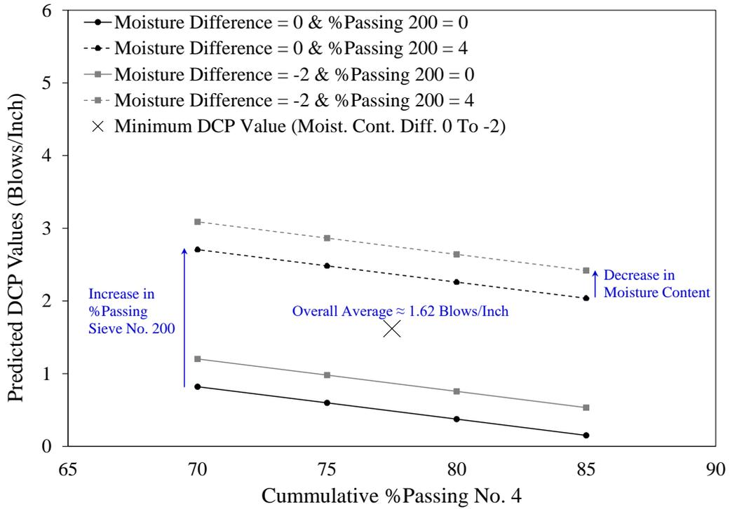
**Figure 13. Example of Computed Minimum DCP Value for NJDOT NAT-1 Aggregates.**
