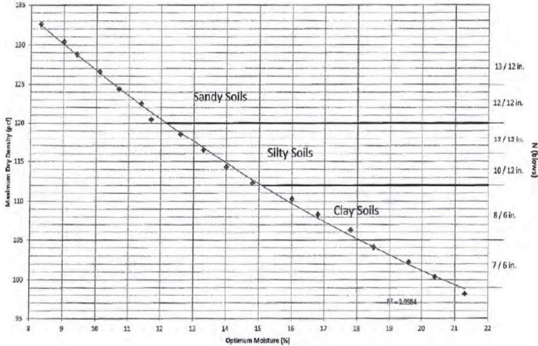
Figure 14. InDOT DCP Acceptance Criteria Based on MDD and OMC of Soil [33].
