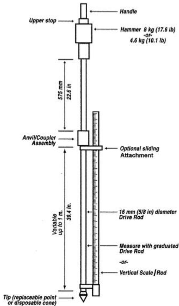
Figure B.1: Assembly Schematic of the DCP [33]
