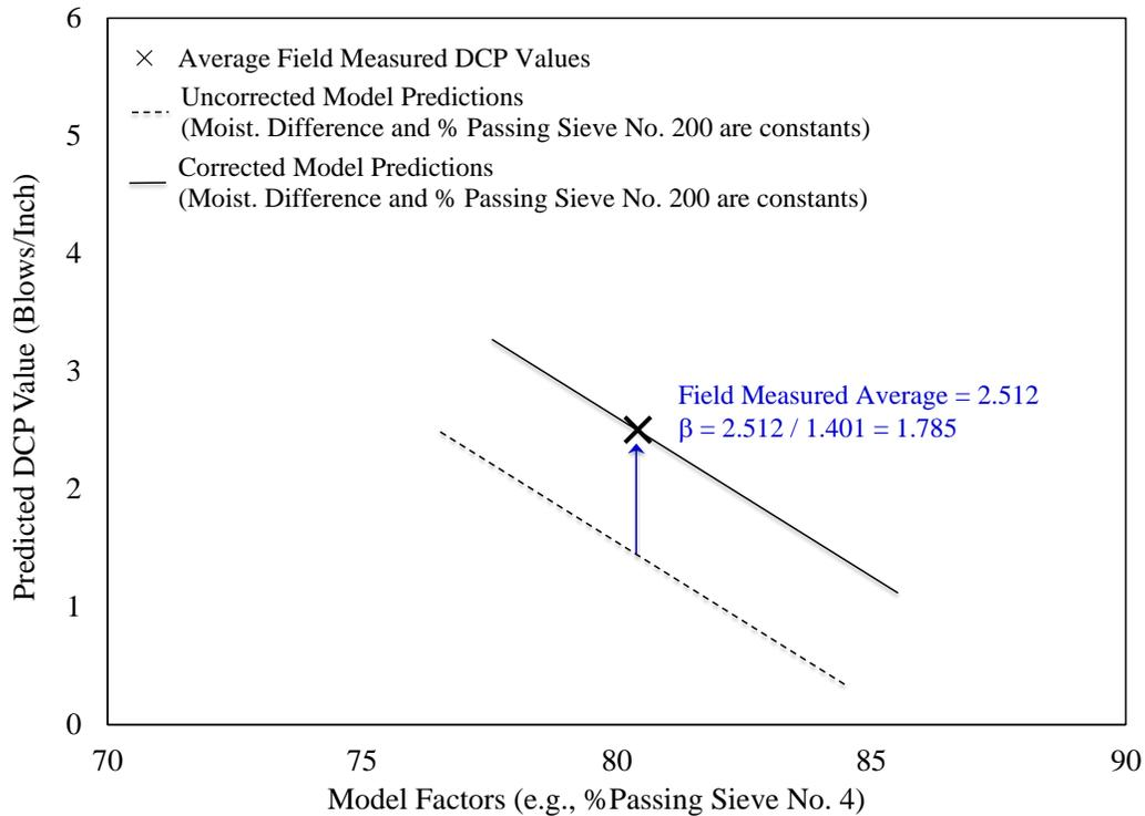
**Figure 12. Computational Procedure Utilized for Computing NAT-1 Aggregates Field Correction Factor.**
