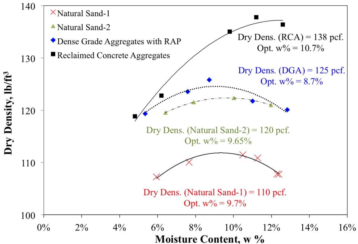
Figure 5. Moisture-Density Relationships for Selected Aggregates.
