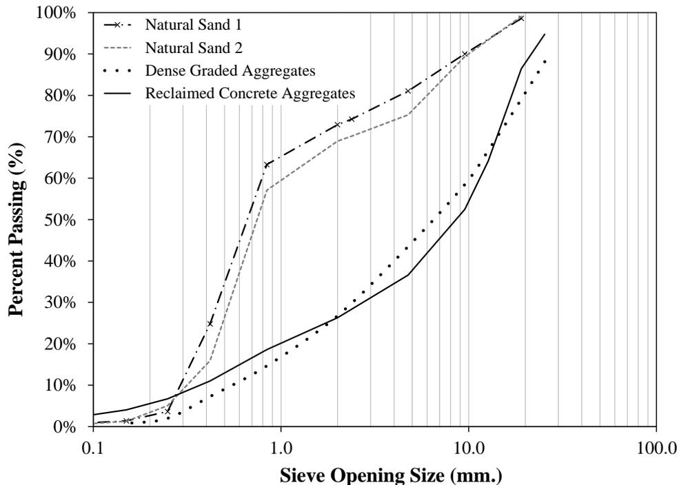
Figure 4. Particle Size Distributions Obtained for Selected Aggregates.
