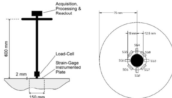
**Figure 1. Initial BCD with Corresponding Plan View of Plate [12].**
