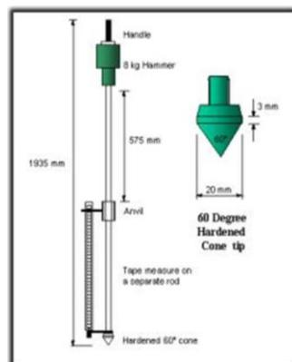
**Figure 3. Schematic of the DCP [6].**
