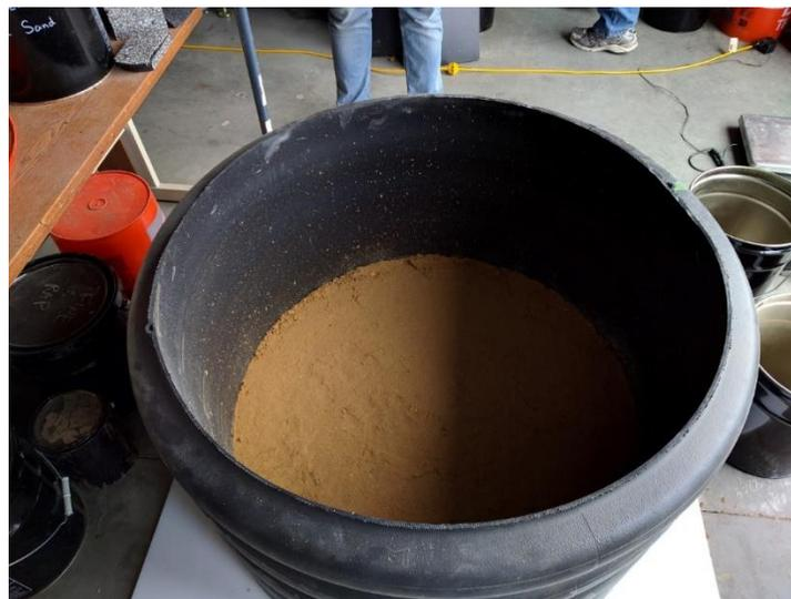
**Figure 10. Large Mold Utilized for Evaluating the Effect of Mold Size.**
