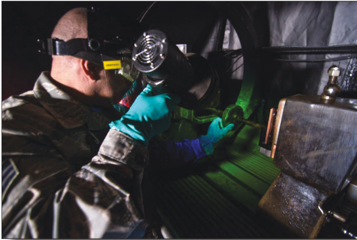
Senior Airman Ray Casanova performs a training exercise of checking aircraft parts under a black light while looking for defects, April 14, 2013, at Atlantic City International Airport. Casanova is assigned to the 177th Fighter Wing Nondestructive Inspection shop. (U.S. Air National Guard Photo by Tech. Sgt. Andrew J. Merlock Jr./Released)
