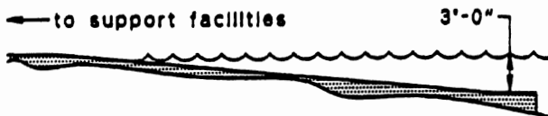
Figure 7.6c Ramp Into Water
