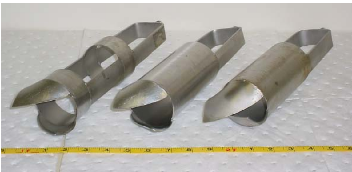
Figure 5.32 Bucket Augers (Photograph by D. Dibblee)
