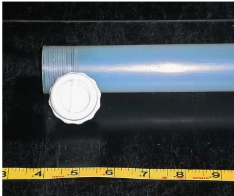
Figure 5.2 Teflon® constructed bailer with Teflon® ball check valve (Photograph by J. Schoenleber)
