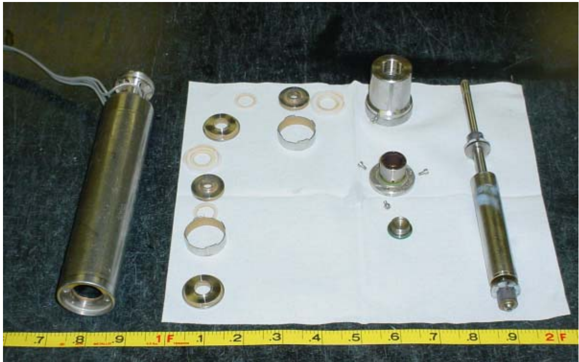
Figure 6.8 Grundfos® Pump being prepared for decontamination (Photograph by J. Schoenleber)
