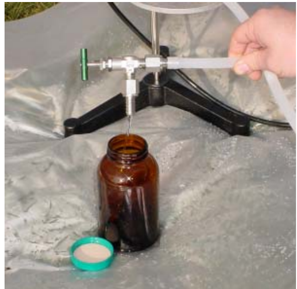
Figure 6.7 Closeup of Needle Valve. (Photograph by D. Dibblee)
