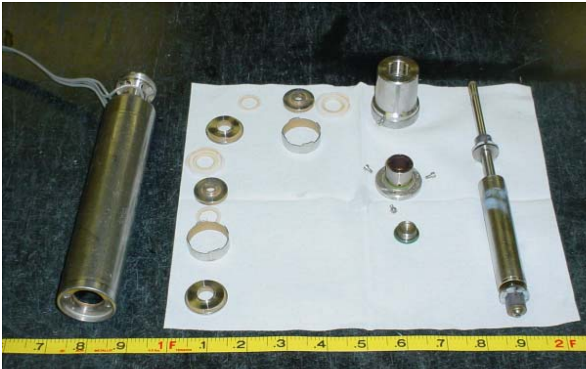
Figure 5.6 Grundfos® Pump being prepared for decontamination (Photograph by J. Schoenleber)
