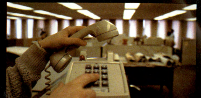
A system of dialing the minimum light needed for office space, under experiment at the World Trade Center, can save up to 50 percent of the electrical energy used in a pre-1973-embargo commercial building.
