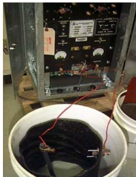
(a) Culvert1-Connected to the Rectifier
