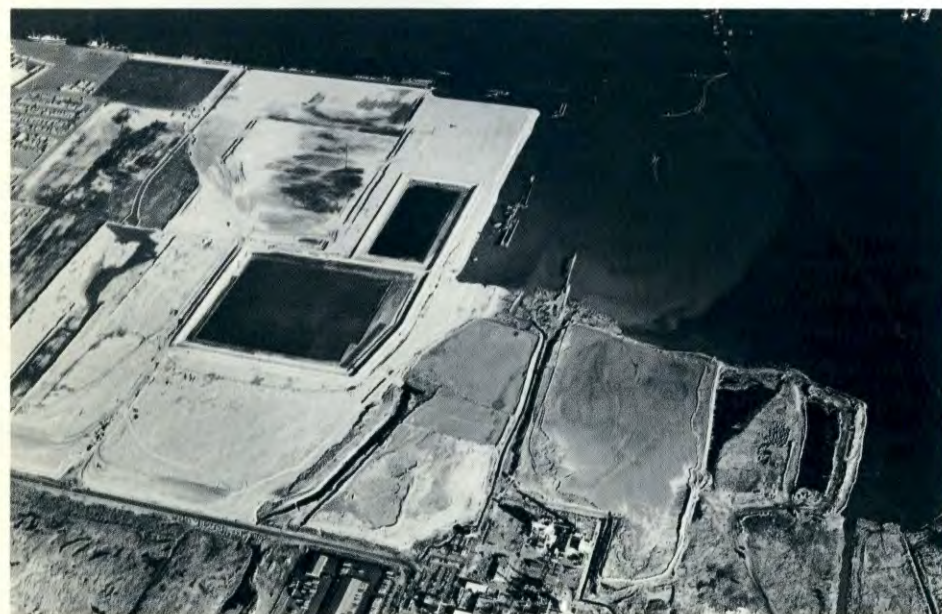
New method of preparing site for construction at the Elizabeth Marine Terminal uses seawater pumped from Newark Bay into huge plastic-lined reservoirs.
