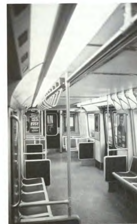
PATH'S newest air-conditioned rapid transit cars have improved seating, additional space at door areas and route indicators above inside doors. The 46 new cars enable PATH to lengthen trains for greater passenger capacity and comfort.
