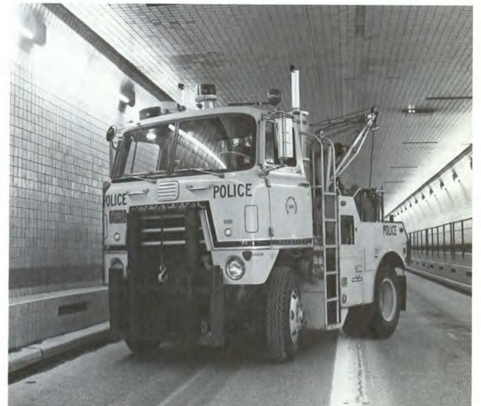
Improved emergency trucks have short turning radius to facilitate removal of disabled vehicles. This is one of 16 such trucks assigned to all tunnel and bridge facilities.
