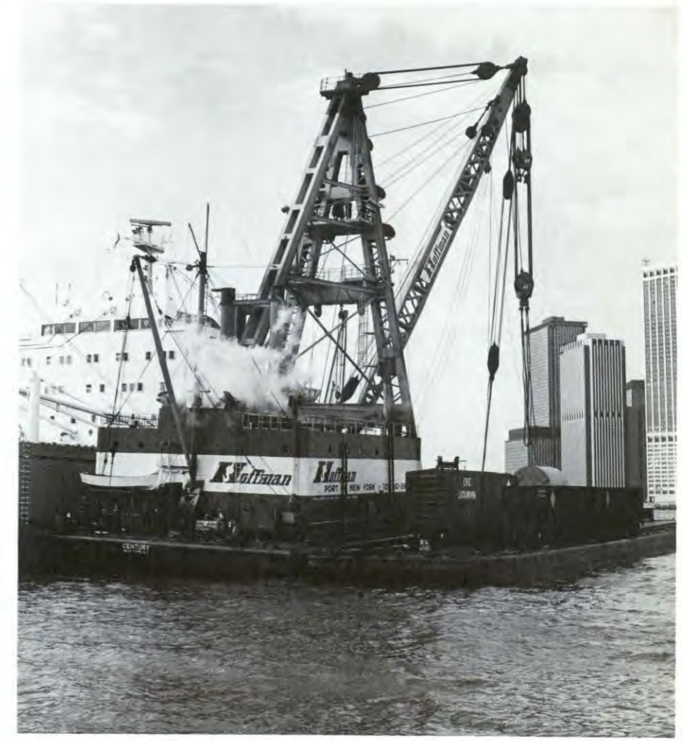
Century, the flagship of the Port Authority's new derrick fleet, prepares to lift heavy cargo from a cartfloat to an outbound ship at the Brooklyn wharfside.
