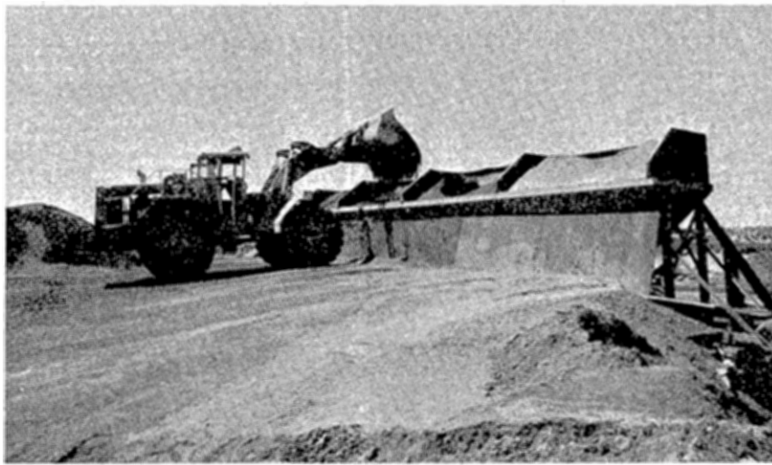
Figure 3: Charging Cold Bins
