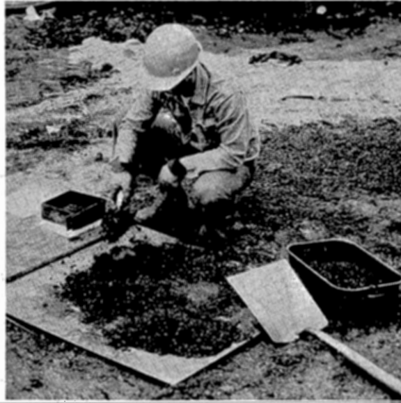
Figure 18: Shaping and Freezing of Asphalt Recovery Samples.
