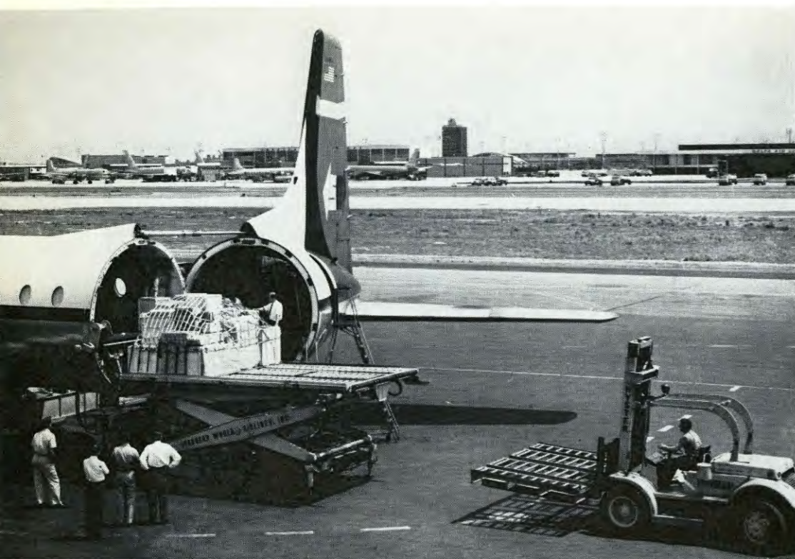
Swing-tail cargo planes speed the handling of shipments at New York International Airport's expanding Air Cargo Center.
