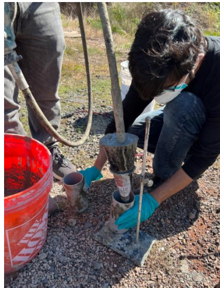
Figure 21. Inverted slump test
