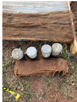
Figure 20. RS flexural and compressive samples curing with burlap
