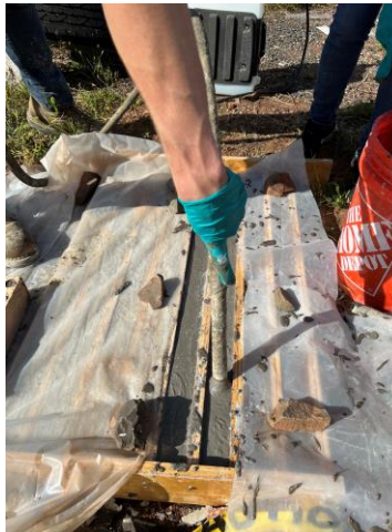
Figure 18. Vibrating the layers of concrete
