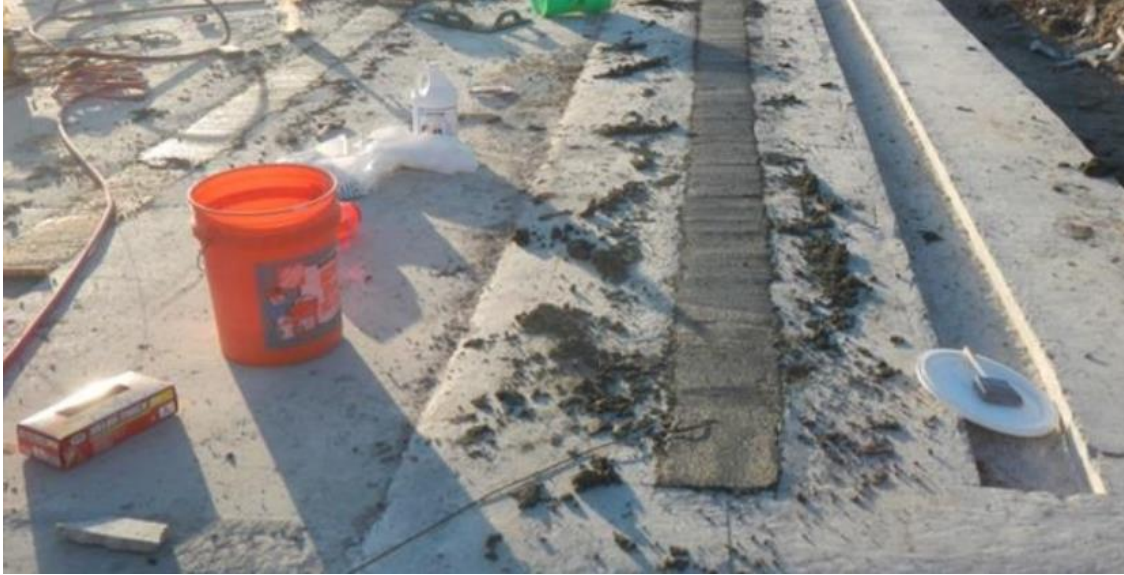
Figure 8. Field test slab with long rectangular defects being repaired similar to partial depth (13)
