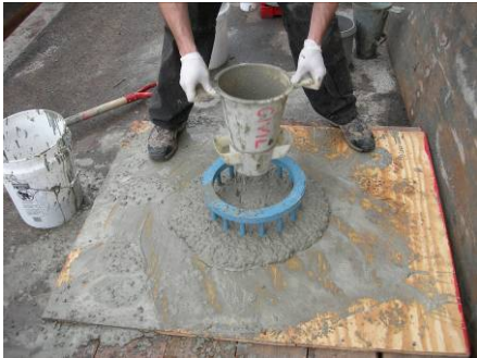
Figure 30. J-Ring Flow Test
