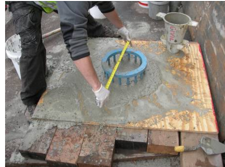
Figure 31. J-Ring Flow Measurement
