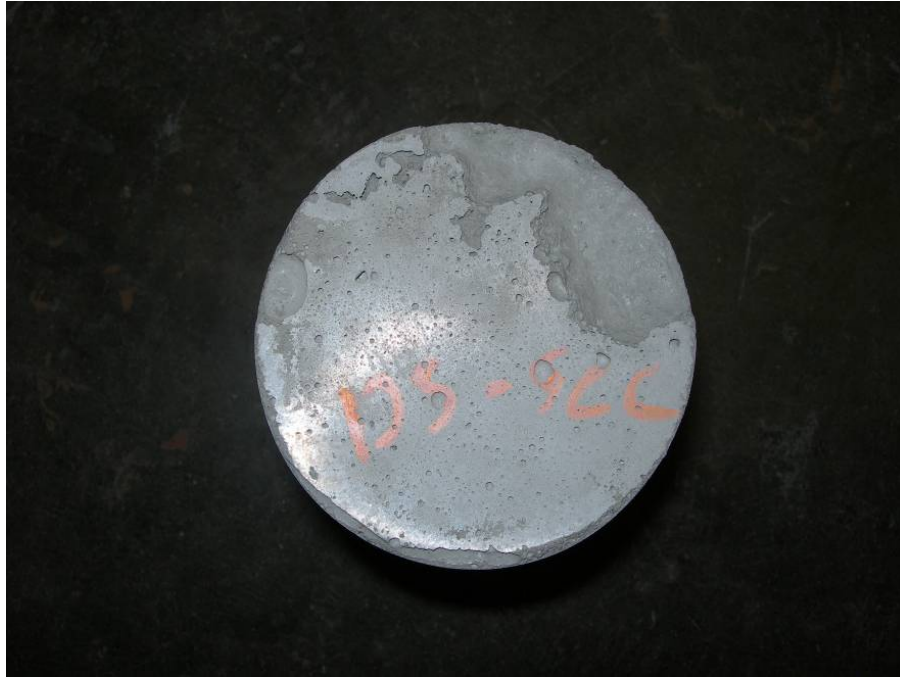
Figure 23. Top View of 6 x 12 inch Test Specimen
