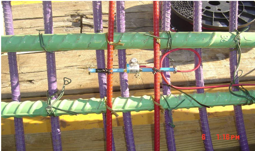
Figure 19. Model 4200 Concrete Embedment Gage
