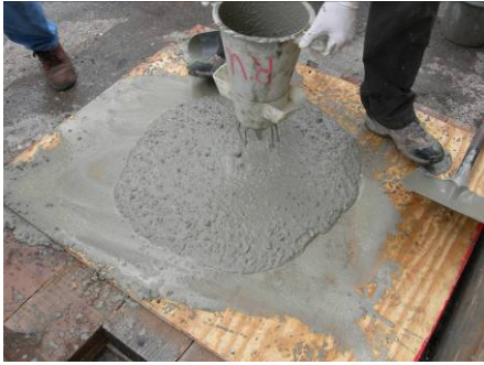
Figure 28. Slump Flow Test
