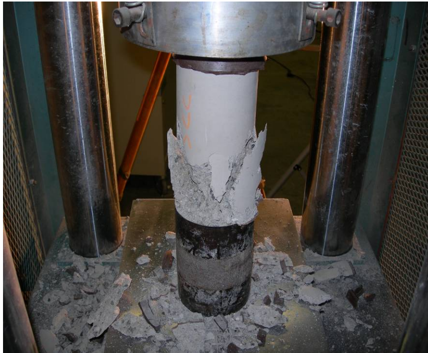
Figure 22. Failure Type of Demonstration Shaft Concrete Under Compression
