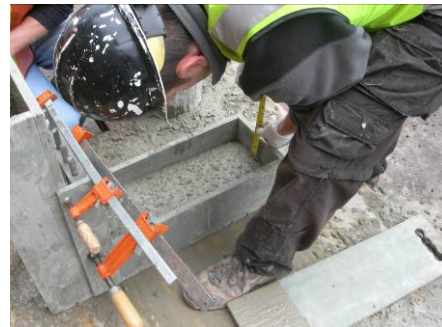
Figure 33. L-Box Test Measurement ( h_2 )
