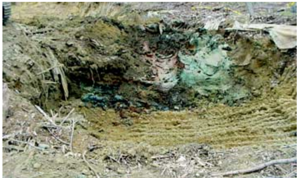
Discolored soil indicates the presence of contamination in the lagoon area.
