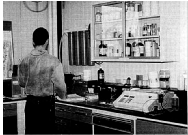
The Manasquan Water Treatment Plant monitors the treated water in its plant laboratory to control the treatment process.
