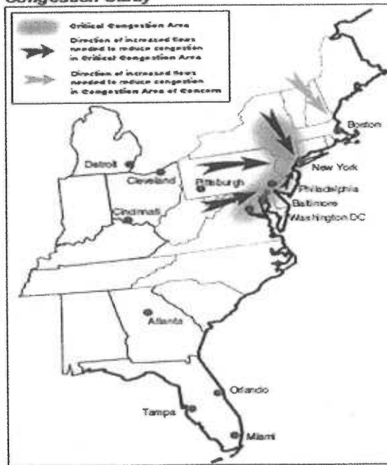
Figure 4-1. Eastern Critical Congestion Area and Congestion Area of Concern Identified in the 2006 National Electric Transmission Congestion Study
