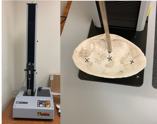
Figure 2: The Instron 3400 Series Single Column Table Model (left) used to measure shell strength (right). Markings on the shell are meaningless.
