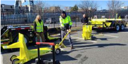
Eight of the 700lb. barriers can be deployed in under 10 minutes by one-person.
