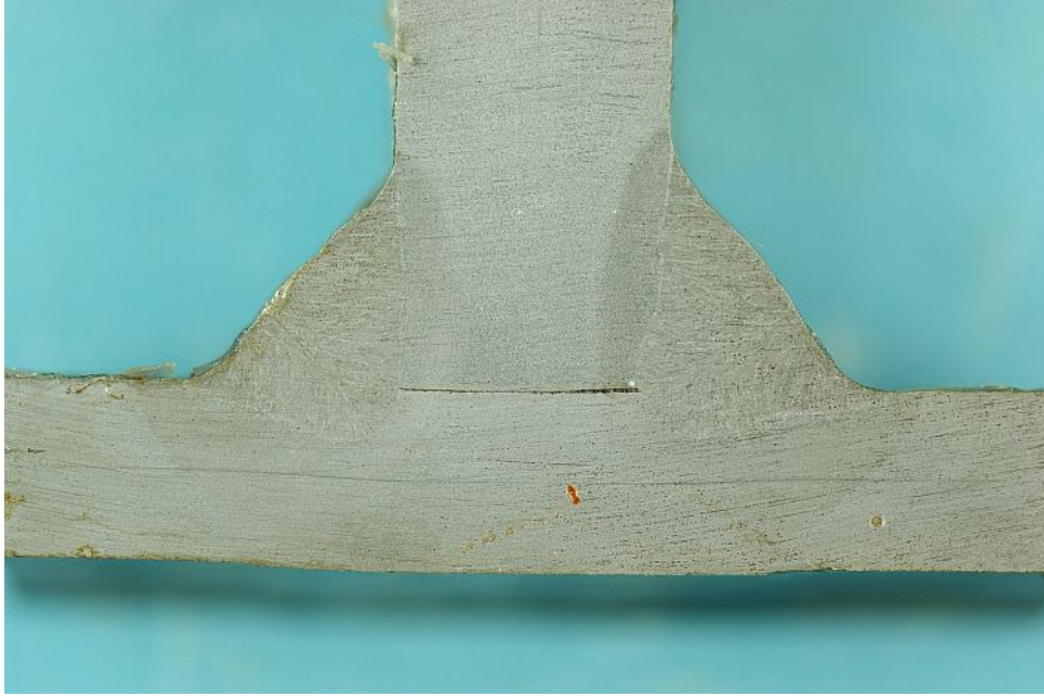
Figure 453. Macro-etched section FS_S_50
