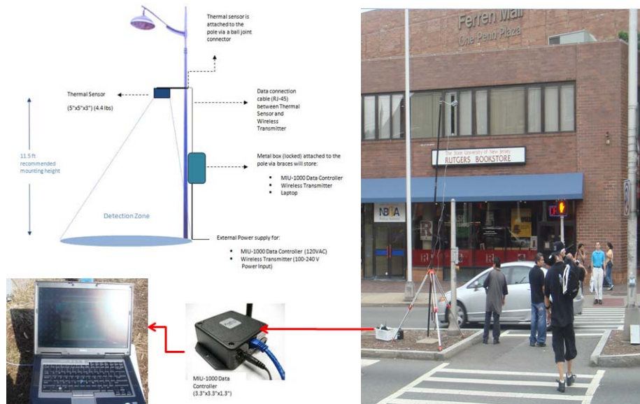
Figure 12. Thermal sensor data extraction
