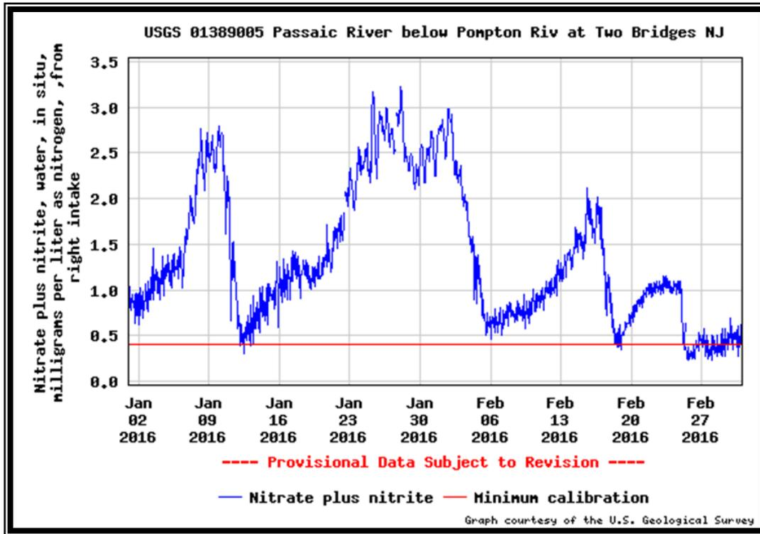
Figure 3. Presentation of continuous nitrate+nitrite data from the right intake at the Two Bridges monitoring station.
