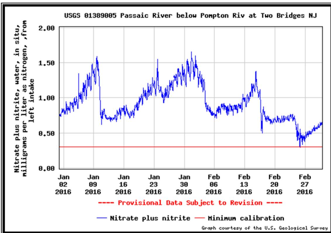
Figure 2. Presentation of continuous nitrate+nitrite data from the left intake at the Two Bridges monitoring station.
