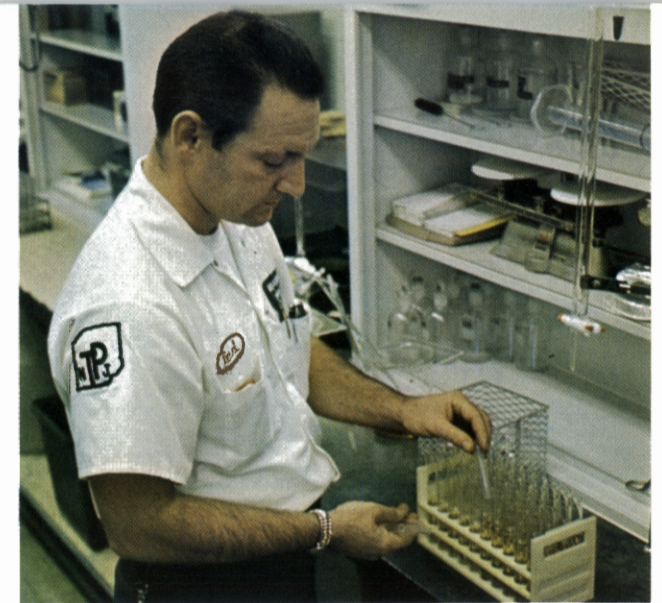
To assure purity of drinking water along entire Turnpike, laboratory technician William Reed sets up culture tubes for bacteriological tests at Hightstown plant.
