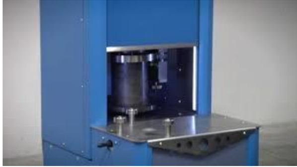
4. ITS breaking head for 6 inch diameter specimens
