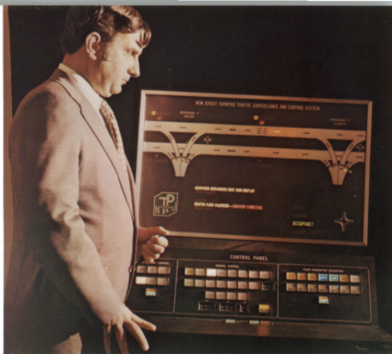
Traffic safety will be enhanced when the computerized surveillance and control system, demonstrated on model above, goes into effect in 1975. The teletype operation (at left) will be incorporated in the new system to detect incidents and change signs for smooth traffic flow.
