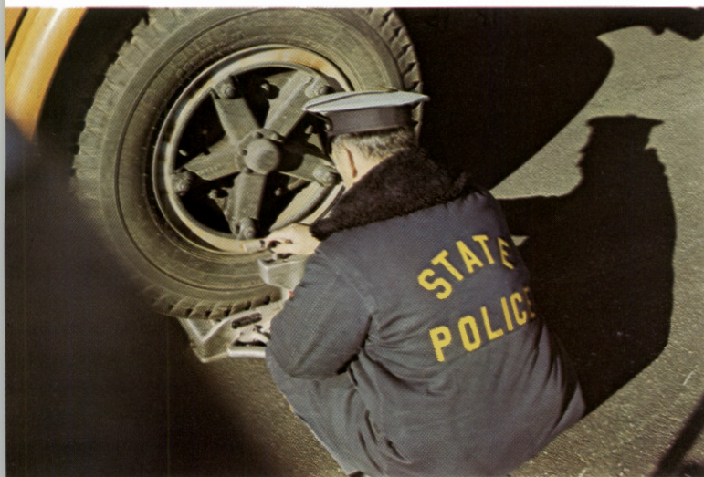
State trooper using portable scale to see that truck load doesn't exceed legal weight.
