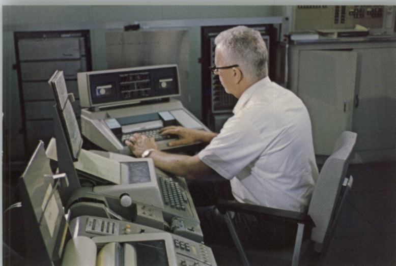
This high speed teletype-writer system, linked to a computer, is capable of changing the speed limits and warning messages on some 84 Turnpike road signs in the northern section at a moment's notice.
