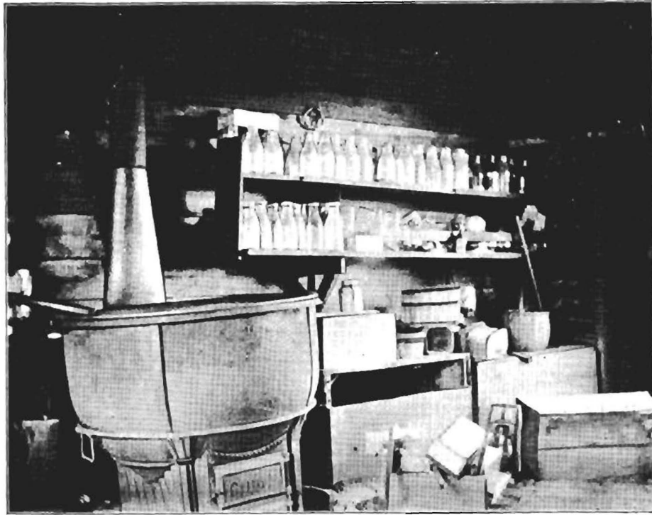
Corner in Bottle-washing Room. Small Pipe over Caldron Connects with Pump about Four Feet Distant.
