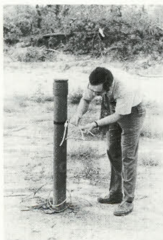
Ground water being checked for movement of pollutants from the sludge.
