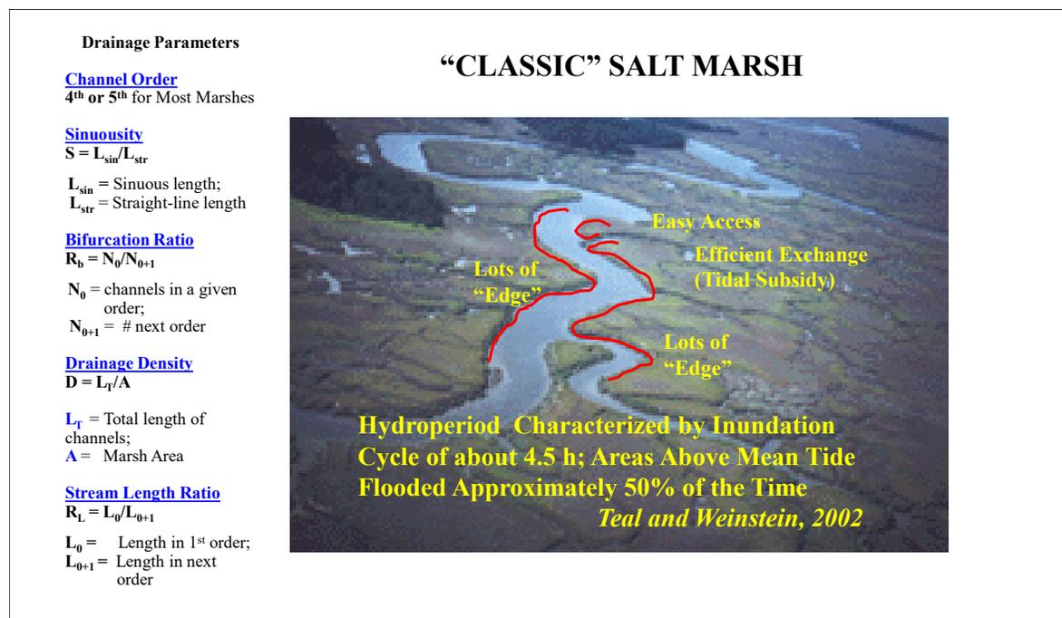
**Figure 7. Salt marsh hydro-geomorphic metrics that can be used to assess the integrity of a wetland complex.**
