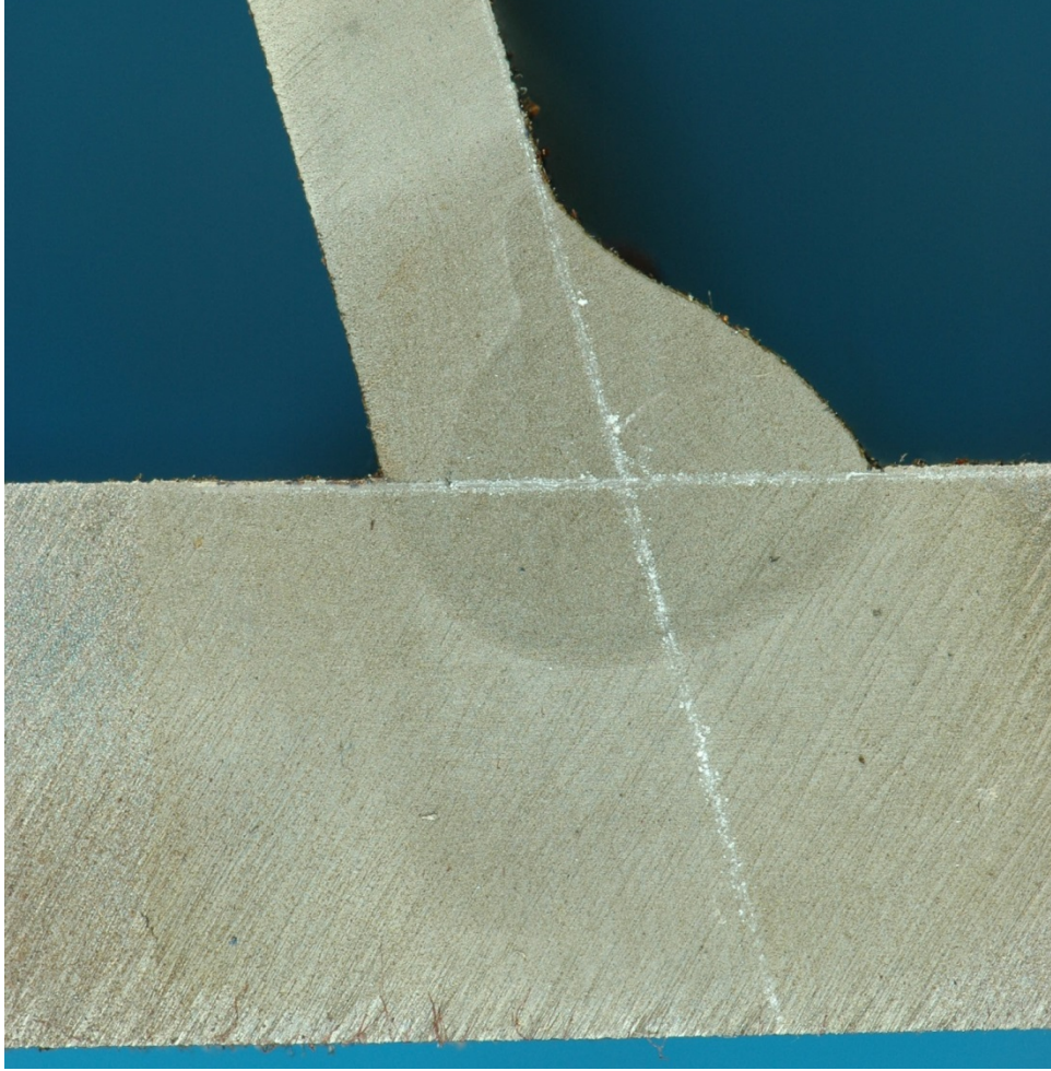
Figure 482. Macro-etched section S34_5
