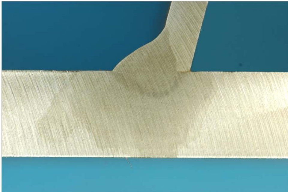
Figure 558. Macro-etched section R2_B_6
