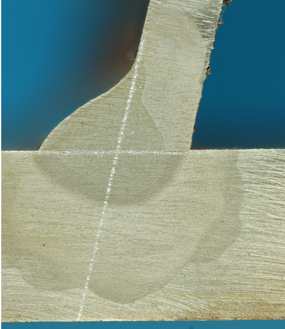
Figure 508. Macro-etched section S34_18
