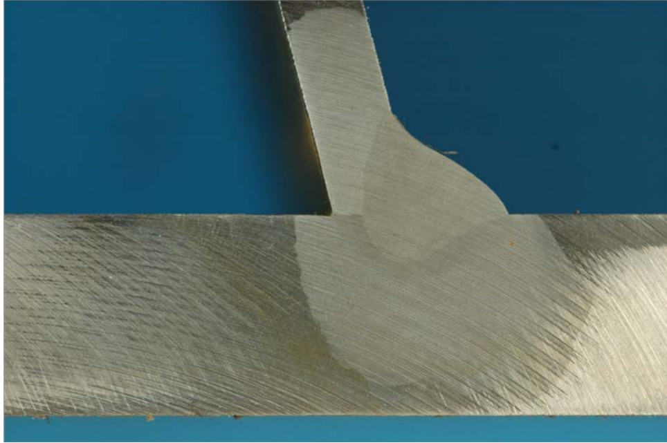
Figure 563. Macro-etched section R2_A_42
