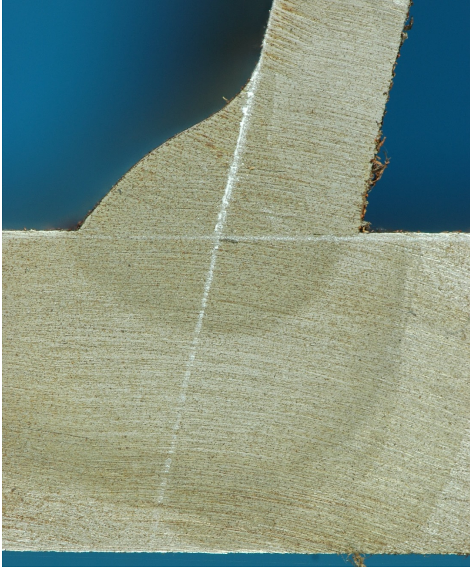
Figure 512. Macro-etched section S34_20
