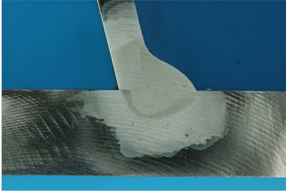
Figure 555. Macro-etched section R1_A_174
