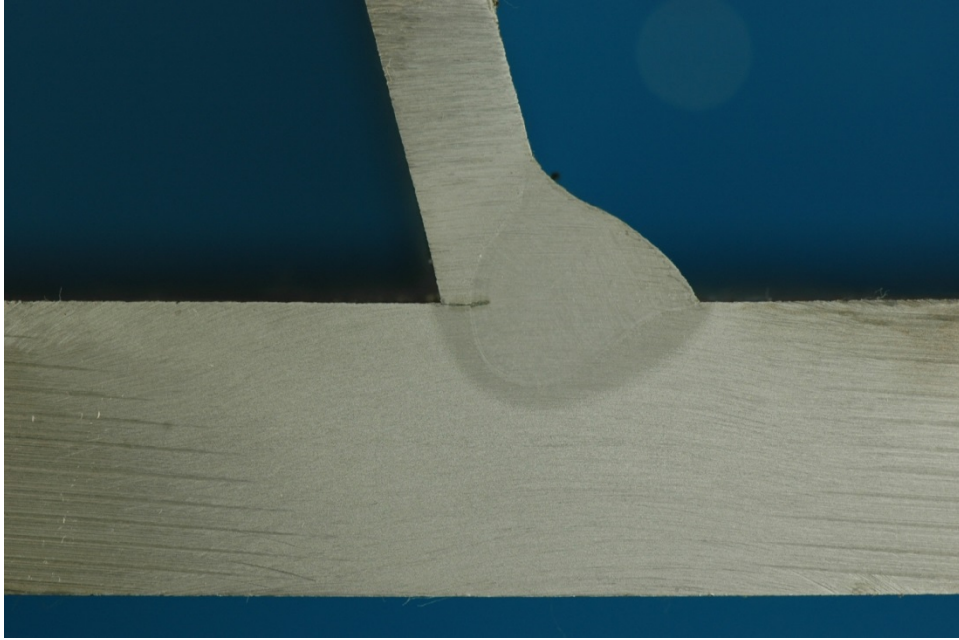
Figure 523. Macro-etched section S12_25
