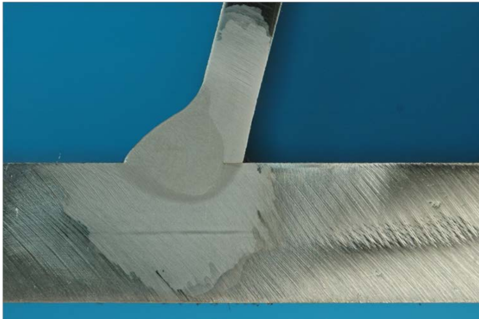
Figure 570. Macro-etched section R2_B_78
