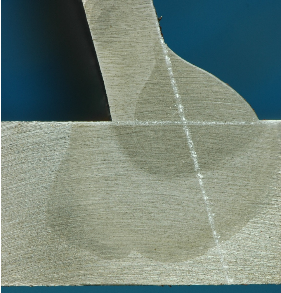
Figure 497. Macro-etched section S12_13
