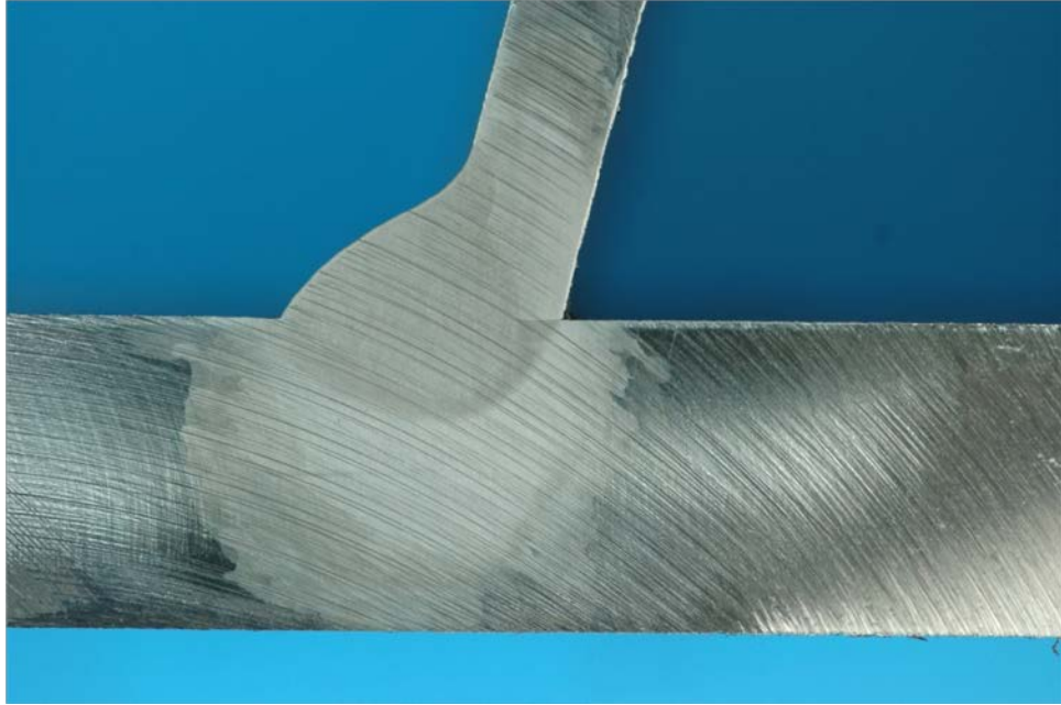
Figure 551. Macro-etched section R1_A_150
