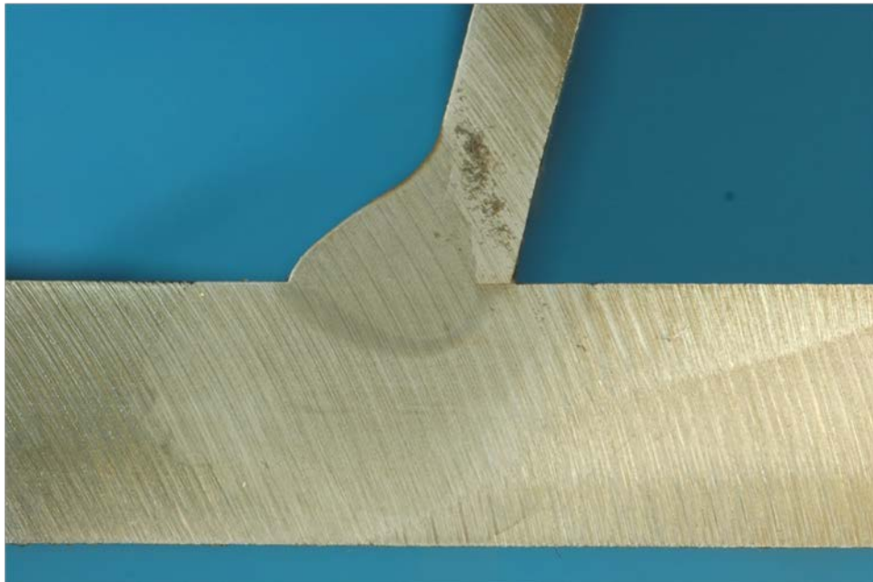
Figure 560. Macro-etched section R2_B_18
