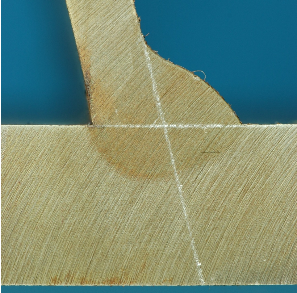
Figure 475. Macro-etched section S12_2
