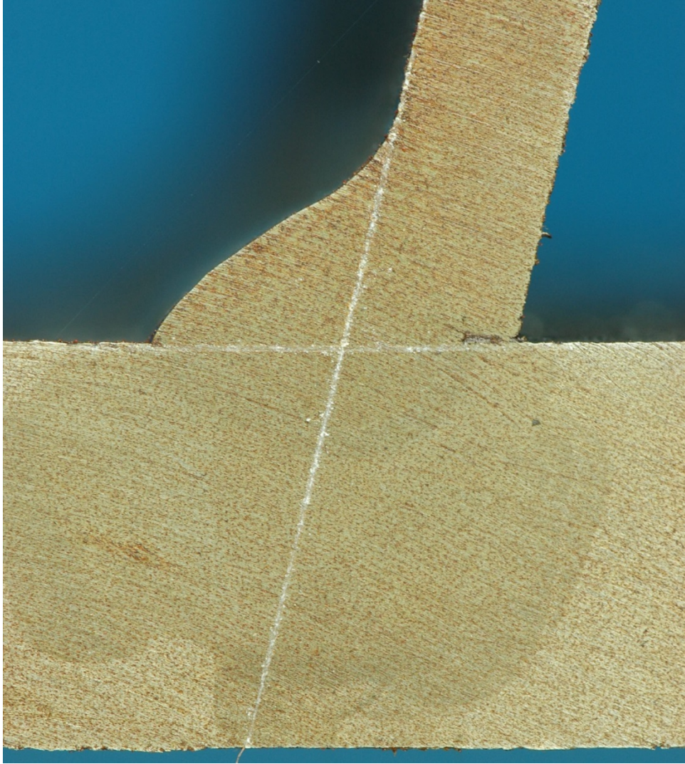
Figure 516. Macro-etched section S34_22
