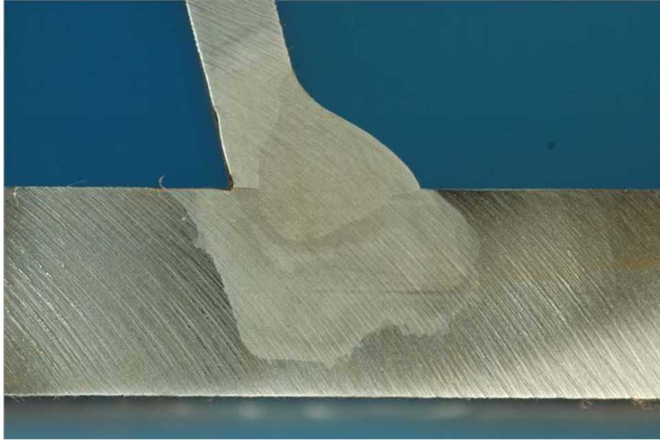
Figure 545. Macro-etched section R1_A_120
