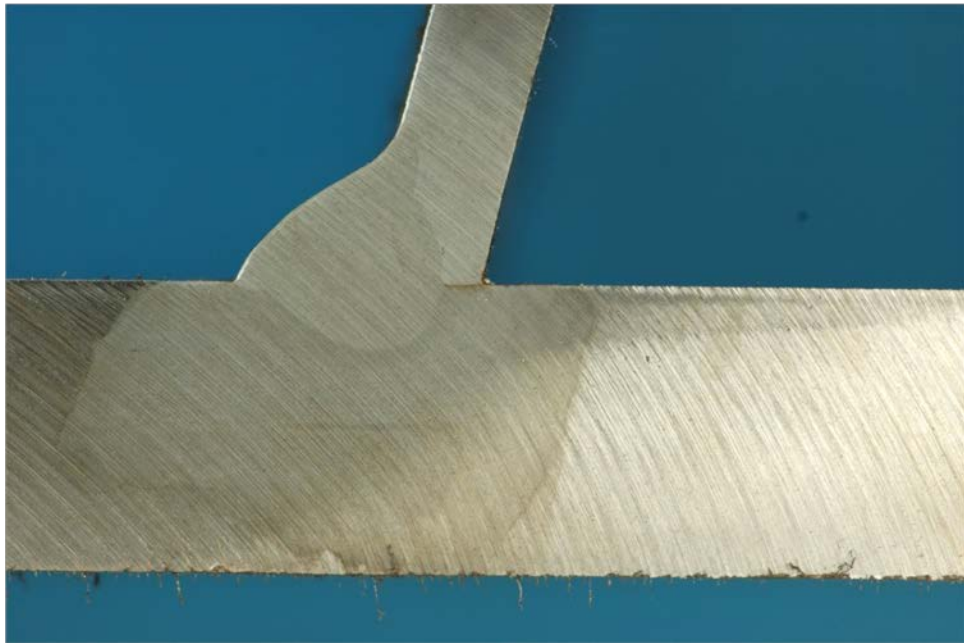
Figure 564. Macro-etched section R2_B_42
