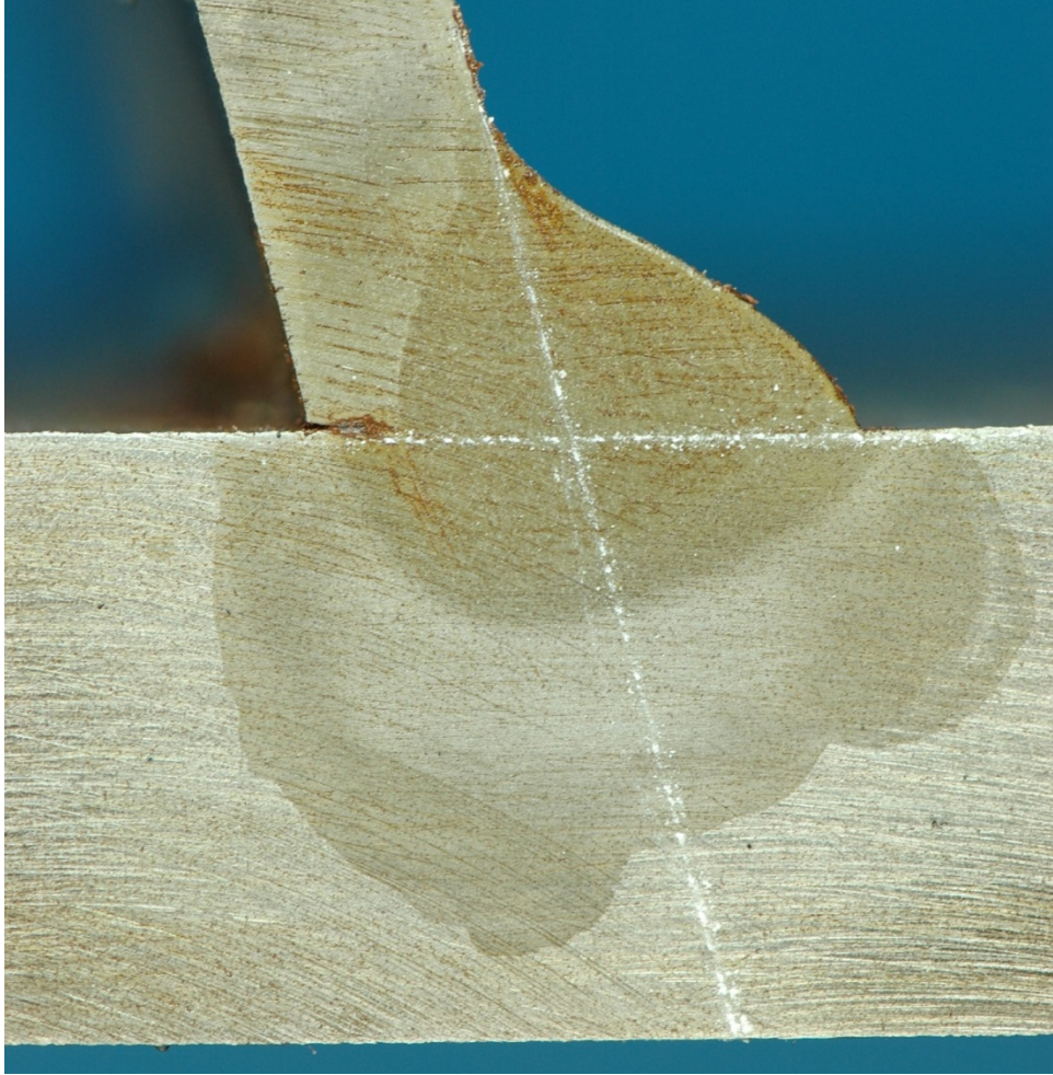
Figure 505. Macro-etched section S12_17
