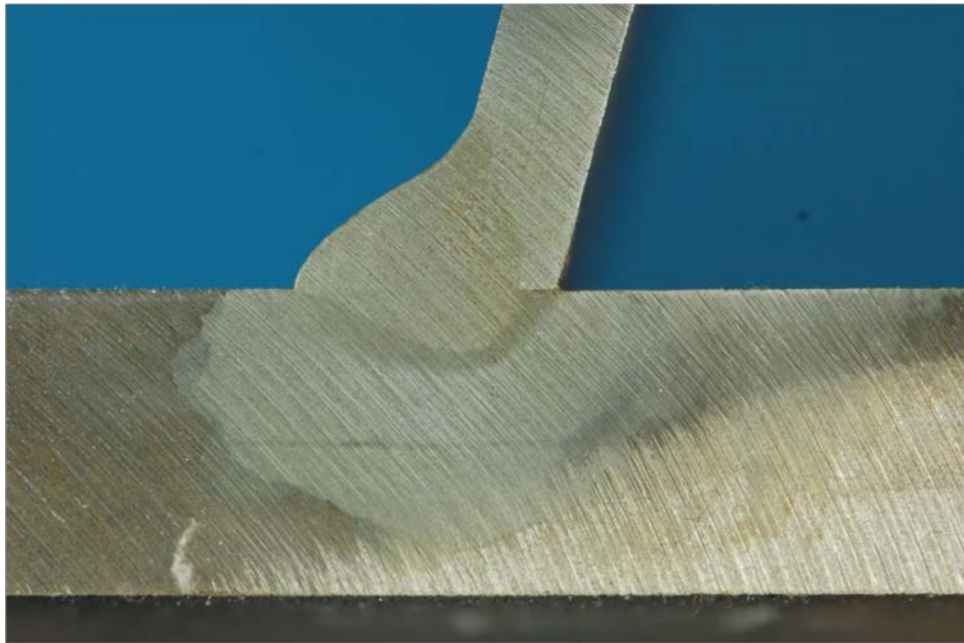
Figure 548. Macro-etched section R1_B_132
