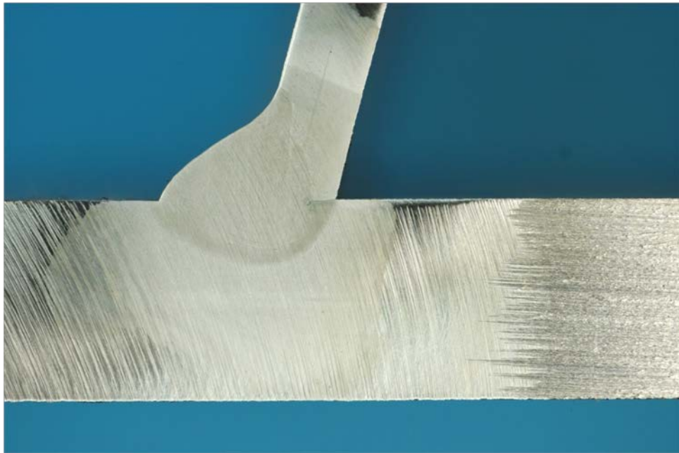
Figure 534. Macro-etched section R1_B_54
