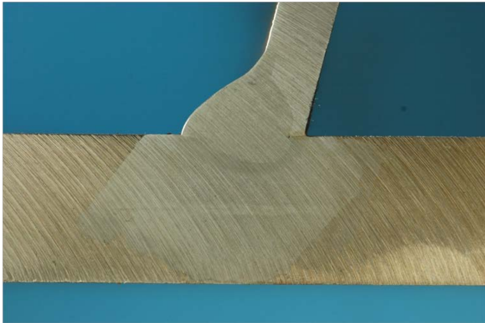
Figure 586. Macro-etched section R2_B_162
