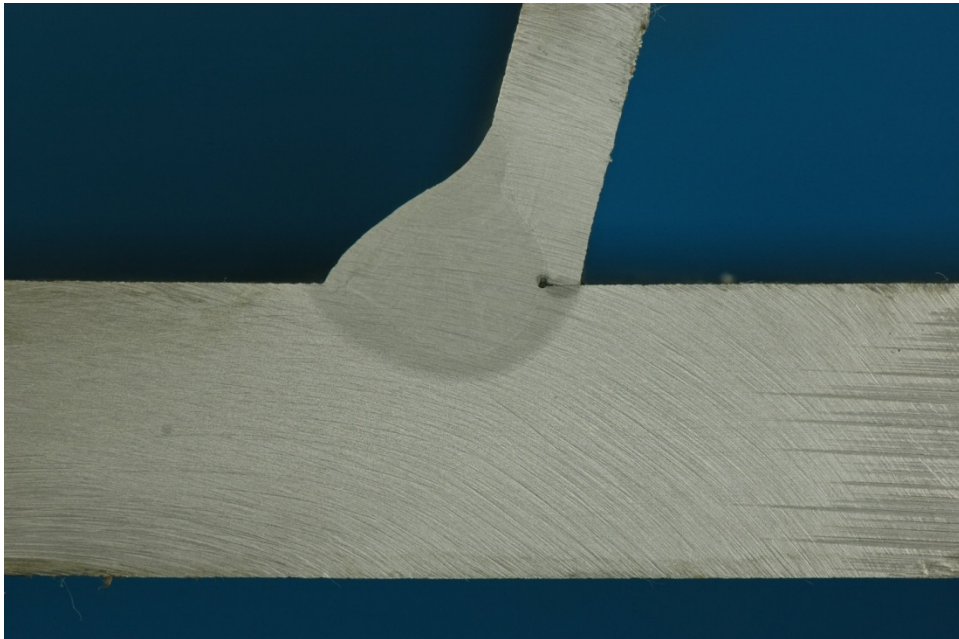
Figure 524. Macro-etched section S34_25
