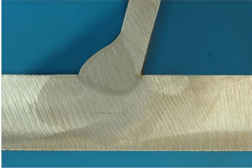
Figure 583. Macro-etched section R2_A_150
