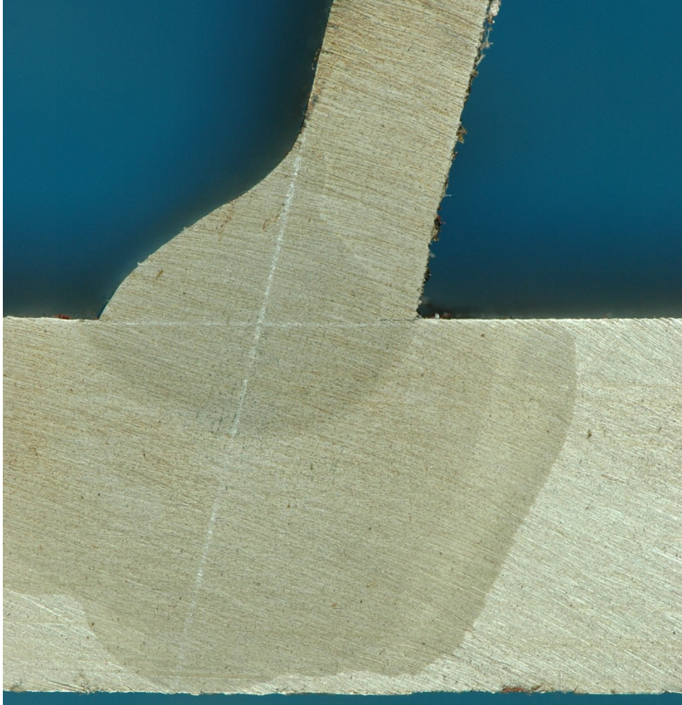
Figure 510. Macro-etched section S34_19
