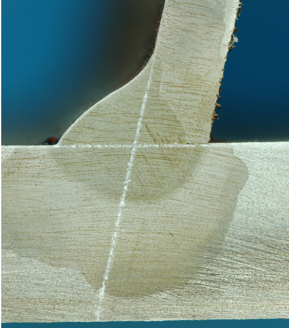
Figure 504. Macro-etched section S34_16
