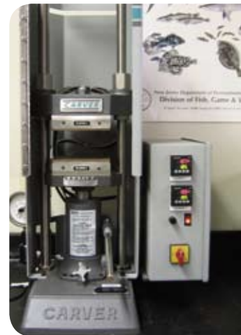
Fish scales are heated in this press to burn an impression onto an acetate slide.
