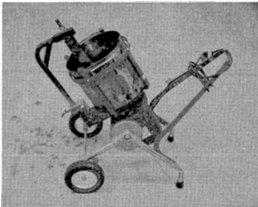
Figure 16 - Rotating 5-gallon Stainless Steel Mixing Bucket
