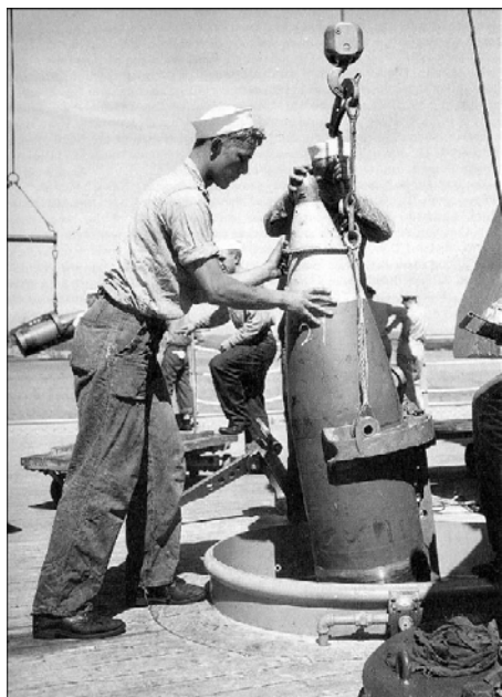
Fig. 10a: Crewmen are seen loading 16" projectiles through a main deck scuttle. The projectiles are hoisted down several decks by a portable beam hoist built onto the top of the main turrets.
