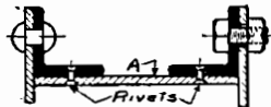
SECTION SHOWING BOLT THREADED INTO ANGLE ONLY - COVER HELD BY NUTS ON ENDS OF BOLTS -
