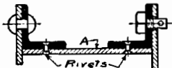
SECTION SHOWING STUD THREADED INTO ANGLE ONLY - COVER HELD BY PINS THROUGH ENDS OF STUDS -
