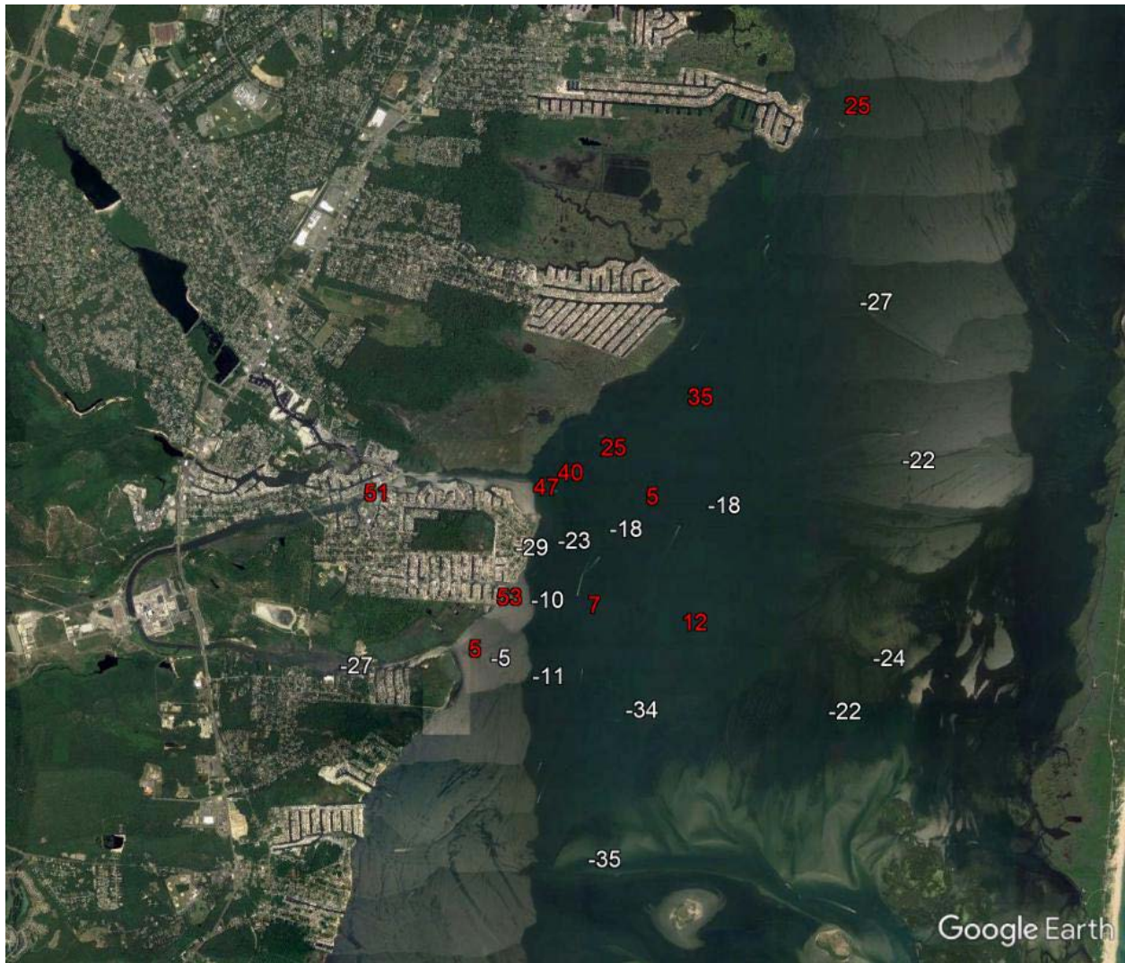
Figure 28. Silt content (percent fraction of total by mass of sediment) anomalies as measured during grab sampling in 2018 prior to OCNCS closure. Red = value above average for all stations, white = value below or equal to average for all stations.
