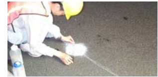
Sand Patch Test
