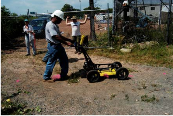
PLATE 7-45: Geophysical Survey Equipment
