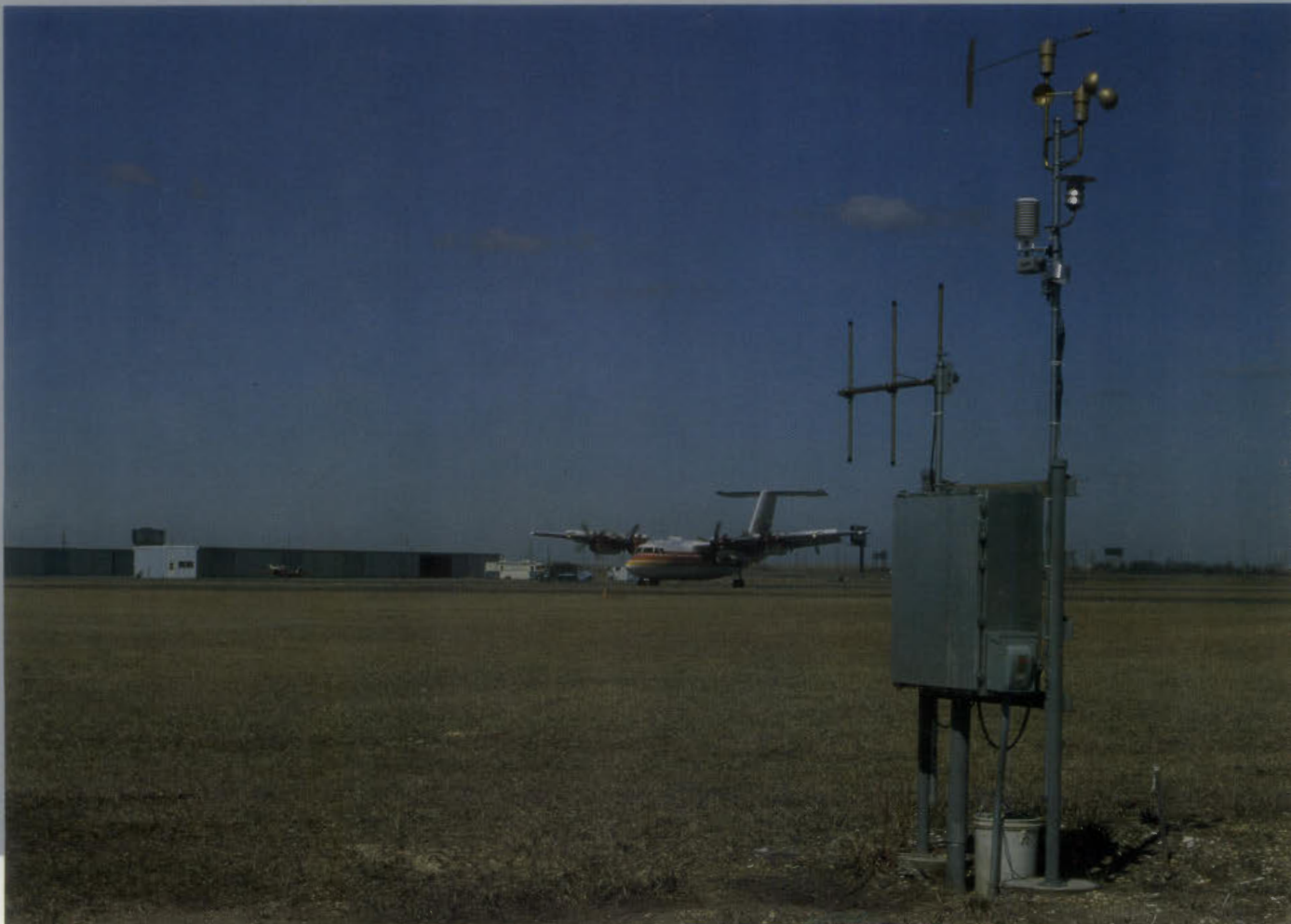
Automated weather observation stations were installed this year at airports statewide, including this one at Bader Field in Atlantic County.
