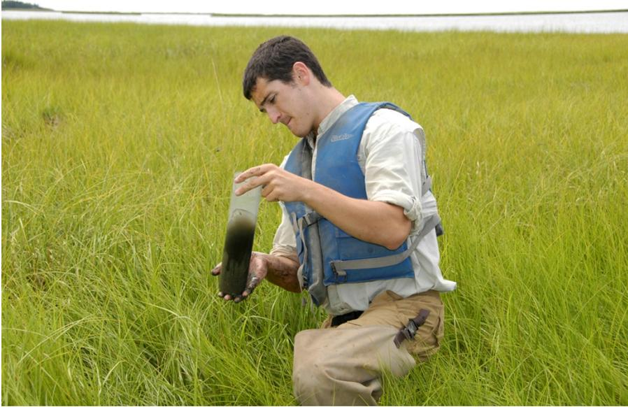
**Figure 2. Collecting sediment samples in wetlands.**
