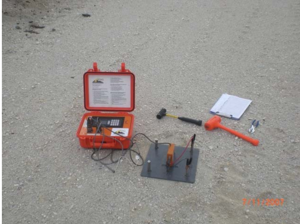
Figure 13 - Electrical Density Gauge (EDG) Setup
