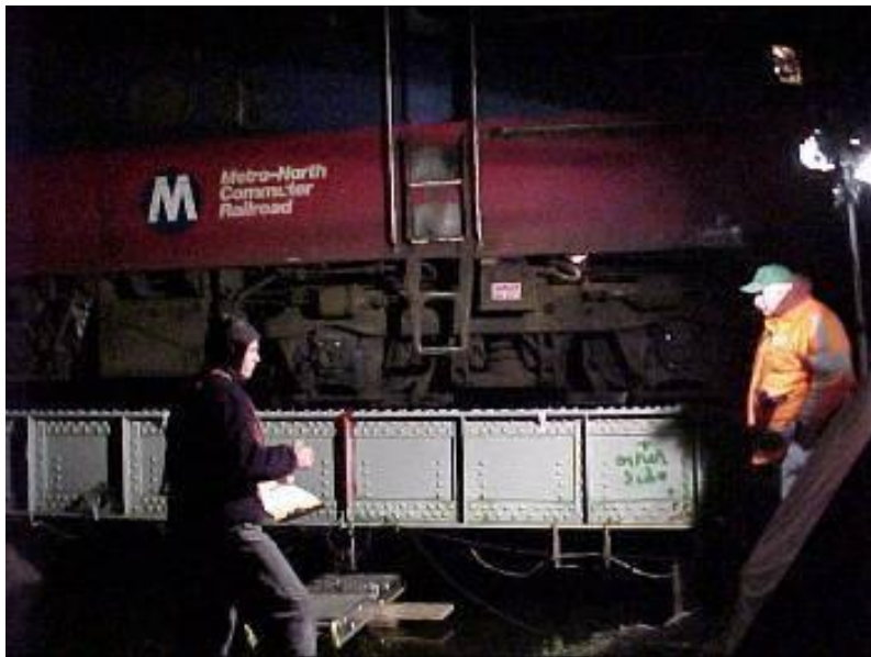
Figure 9. Train positioned for static test (11)
