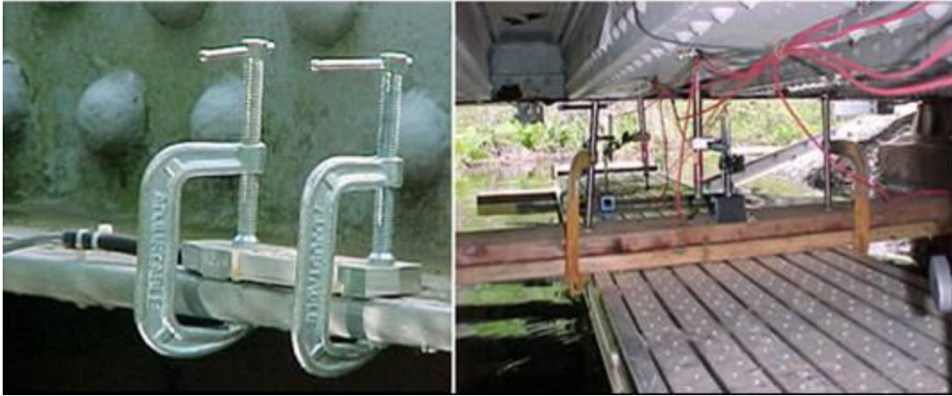
Figure 8. Sensors used to measure strains and deflection (11)
