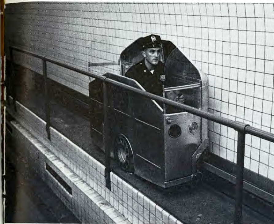
Traffic control improvements studied during the year at Port Authority vehicular crossings included the catwalk car now being tested in a portion of the South Tube of the Lincoln Tunnel. The unique vehicle travels rapidly in either direction to help officers expedite the movement of traffic.
