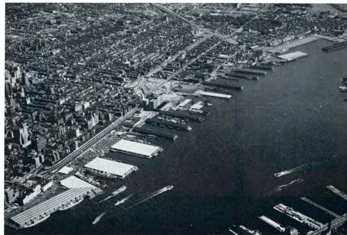
This aerial view from Manhattan of the Brooklyn waterfront shows steamship activity at the Brooklyn-Port Authority Piers. The $90,000,000 redevelopment program for this two-mile stretch of prime waterfront, begun in 1956, will be completed in 1963. It includes construction of 11 new piers, rehabilitation of an existing pier and improvement of 49 upland acres.
