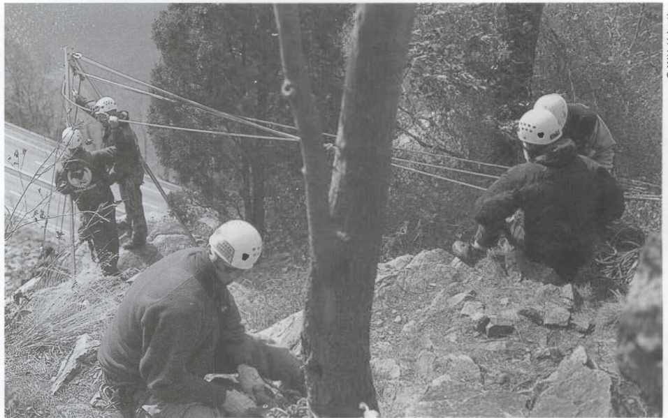
A hauling system, utilizing mechanical advantage provided by ropes and pulleys, is set up to lift a load up the cliff face.
