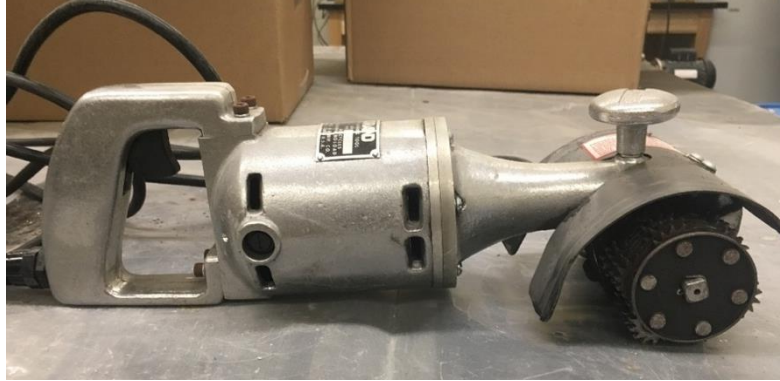
Figure 6. Aurand hand-held steel toothed cleaning machine
