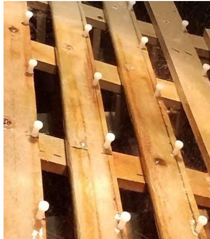
Figure A7. Shoulder Screws Installed on the Specimen Holding Rack to Prevent Slipping
