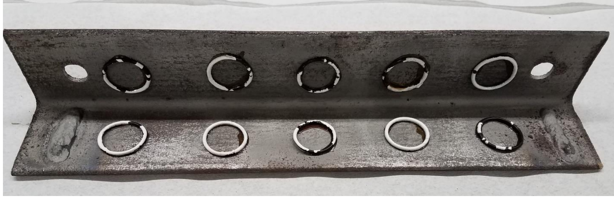
Figure 10. O-rings attached to steel specimen
