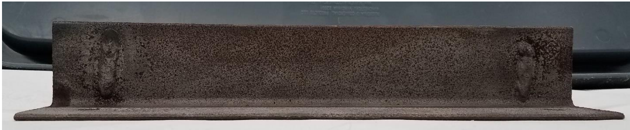
Figure 9. Typical 1-inch-long welds on steel specimens
