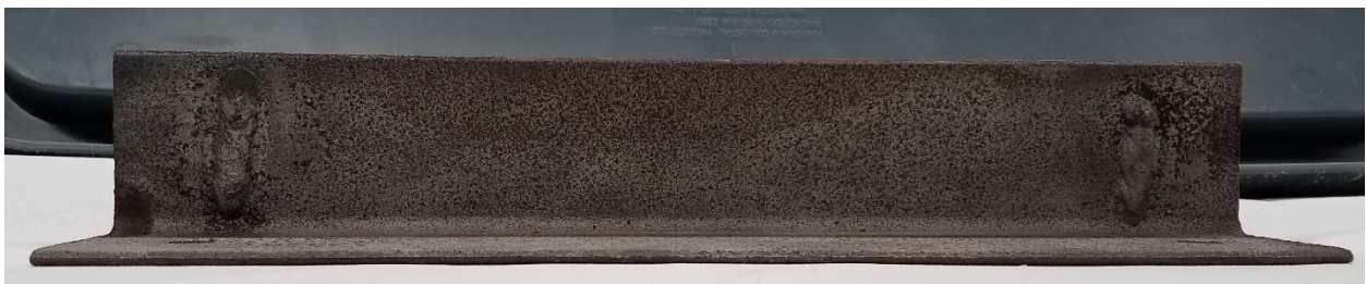
Figure B2. Typical 1-inch-long welds on steel specimens
