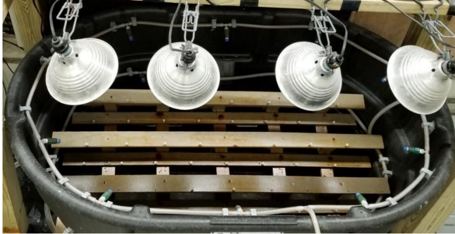
Figure 1. Chamber for Accelerated Testing: Salt Sprayers and Holding Rack
