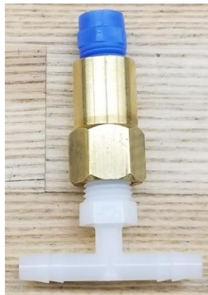
Figure A5. Salt-Water Sprayer Assembly
