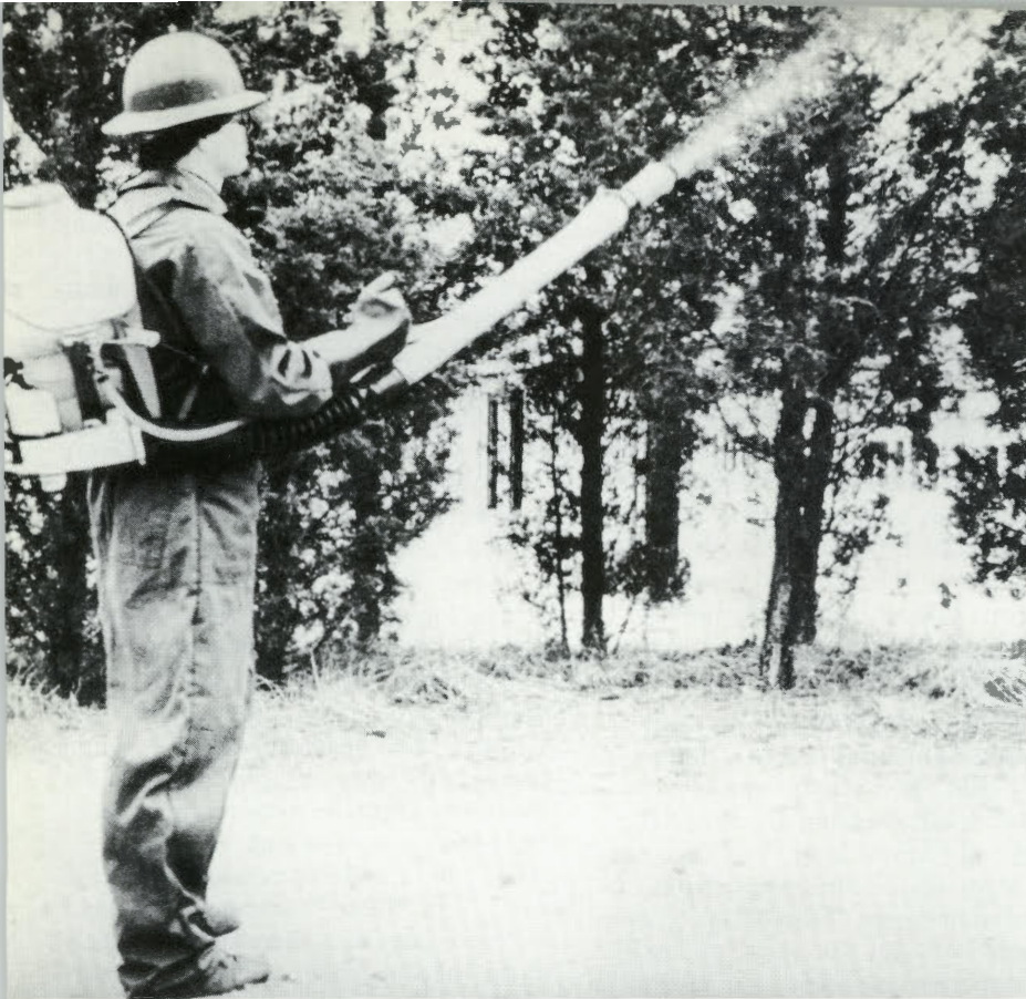
A back-pack, motor driven sprayer in operation.
