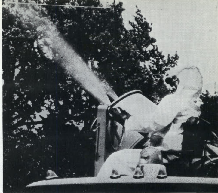
A large mist blower in operation mounted on a flat bed truck for road side spraying.
