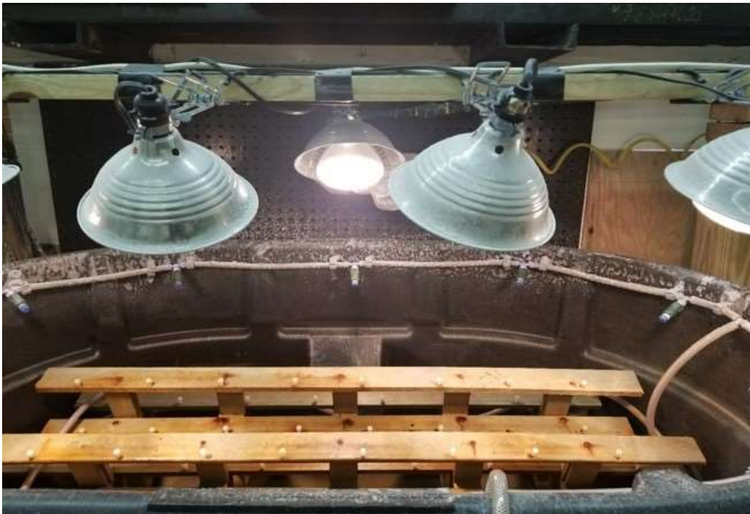
Figure 35. Corrosion equipment using UV at Rutgers University
