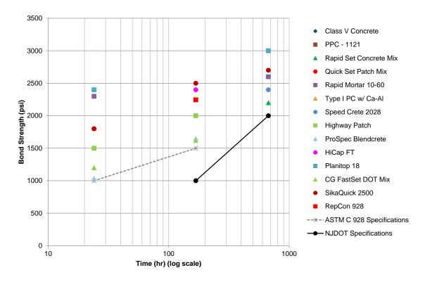
Figure 24: Bond Strength of CIP Mixes
