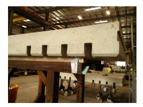
Figure 10: Fort Miller bottom-slot dowel system.
