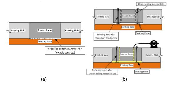
Figure 9: Precast panel support methods. (From Tayabji, 2016a).
