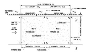
Figure 5: Schematic for determining lay length (NPCA, 2017).
