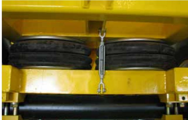
*Figure 47. Turnbuckle Supporting Axle and Swingarm.*
