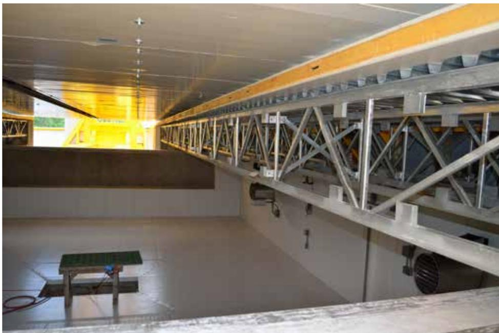
*Figure 34. Lower Environmental Chamber Showing Foam Lining.*
