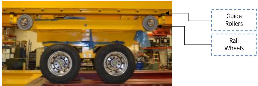
*Figure 13: Side View of the Carriage Assembly Highlighting the Rail Wheels and Guide Rollers*
