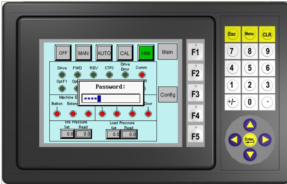
Figure 37. HMI Password Screen.
