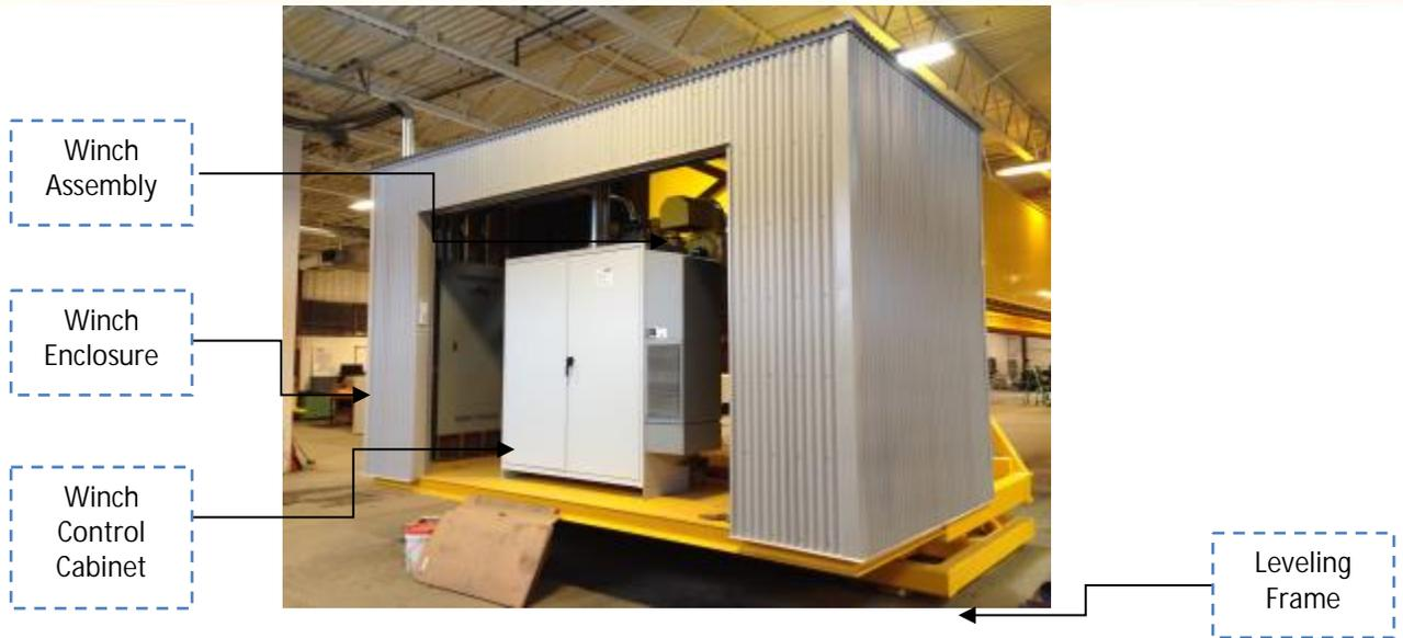
*Figure 3. Winch End Frame Assembly Showing Winch, MDP, and Winch Controller*
