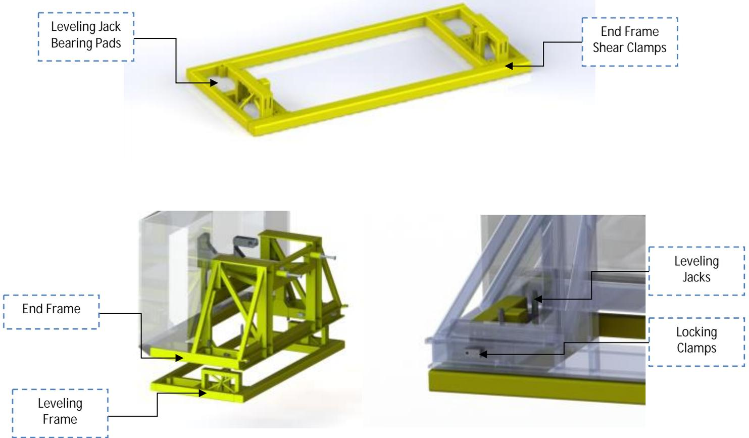
*Figure 5. Leveling Frame Assembly*
