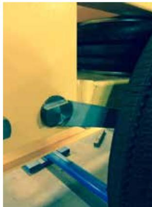
*Figure 46. Axle Alignment Fixture in Place on One Side of Carriage.*
