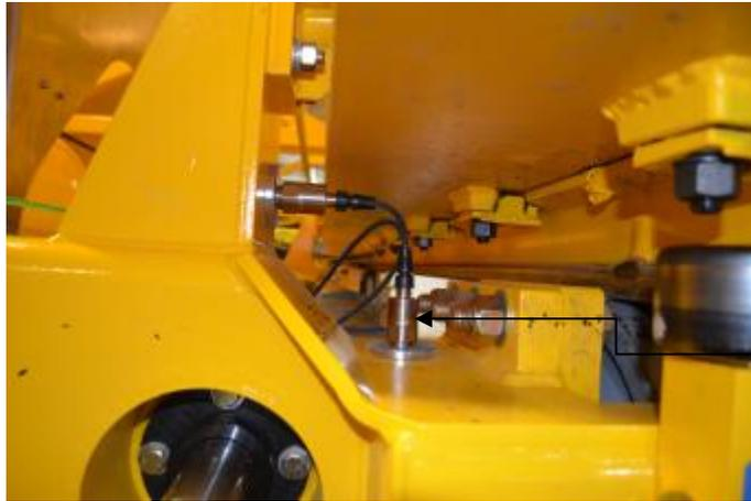
*Figure 15: Vibration Sensors located on the Upper Carriage Assembly.*
