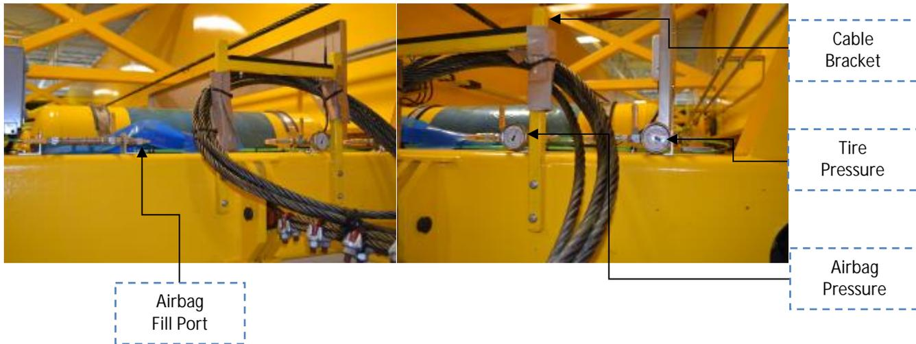
*Figure 14: End View of the Upper Carriage Assembly Highlighting Pneumatic items.*
