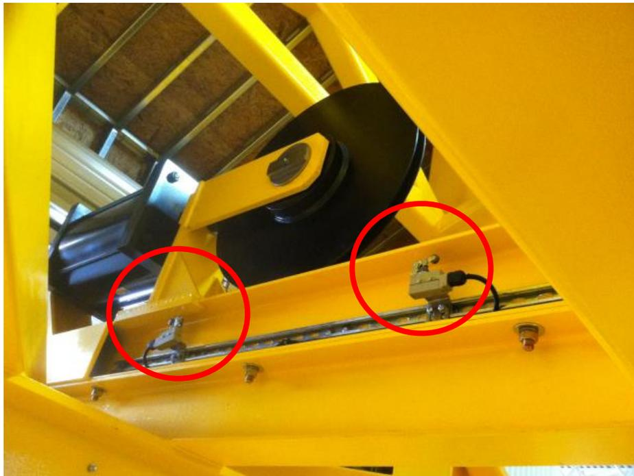
*Figure 25: Tension cylinder with cylinder extend and retract switches (circled)*
