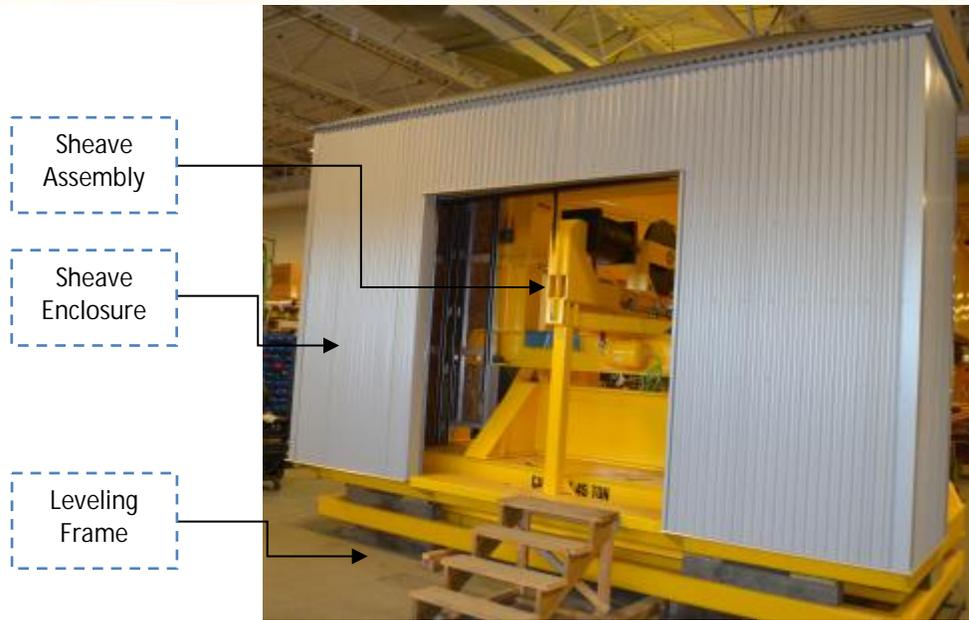
*Figure 2. Sheave End Frame Assembly*
