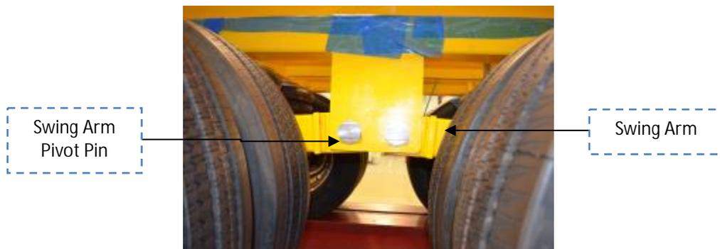
*Figure 20: Side View of the Lower Carriage Assembly Showing the Swing Arms and Pivot Pins.*
