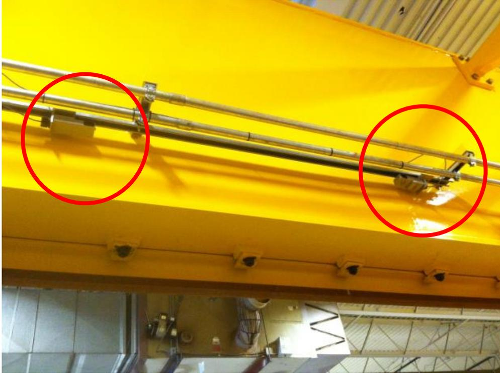
*Figure 24: Optical limit switches (circled).*
