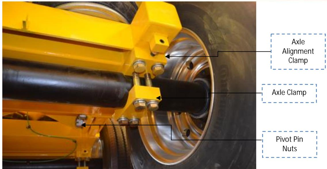
*Figure 21: Bottom View of the Lower Carriage Assembly Highlighting the Axle Clamp and Alignment System.*
