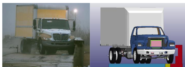
Figure 2. Crash test and simulation comparison at collision for single unit truck
