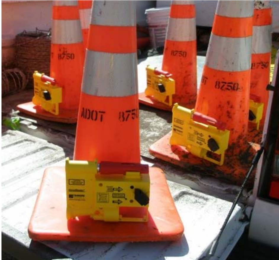
Figure 1. Close-Up of SonoBlaster! ® Work Zone Intrusion Alarm.
