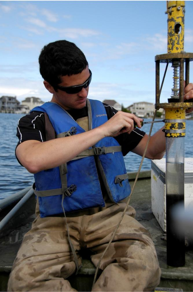
**Figure 4. Collecting sediment samples in open water with a Glew corer.**
