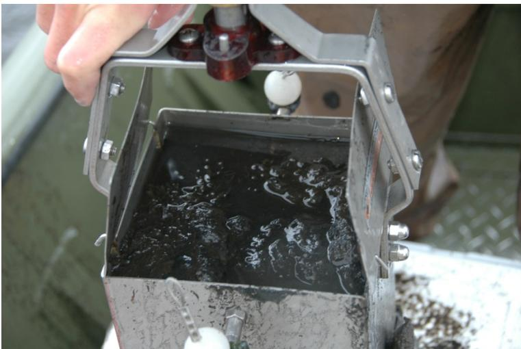
**Figure 5. Collecting surface sediment sample with an Ekman Grab sampler.**
